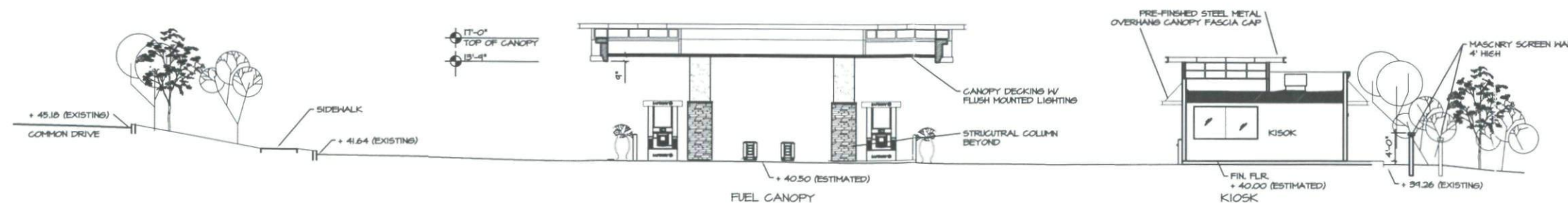
1 SITE SECTIONS - EAST WEST SCALE: 1/8" = 1'-0"
