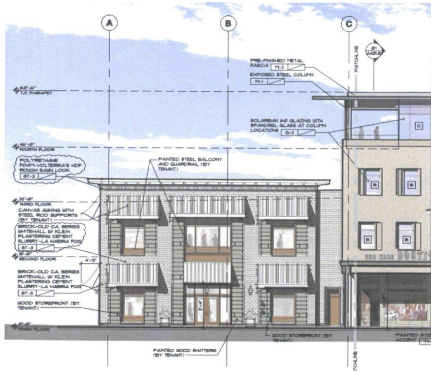
01 BUILDING B PARTIAL WEST ELEVATION SCALE: 3/32" = 1'-0" REF:
