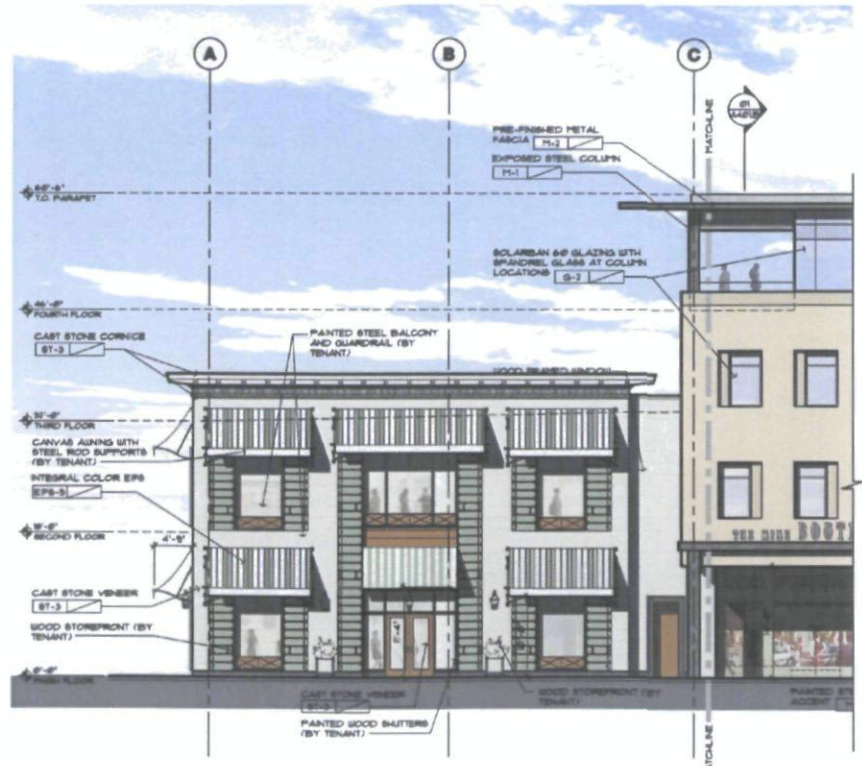
BUILDING B PARTIAL EAST ELEVATION - 01 - SCALE: 3/32" = 1'-0" REF:
