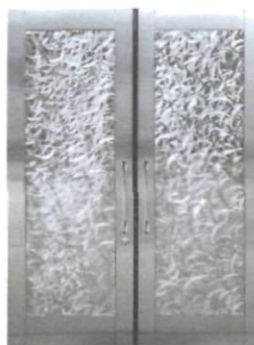
Single inset stile & rail: satin finish stainless steel. Insets: random finish stainless steel
