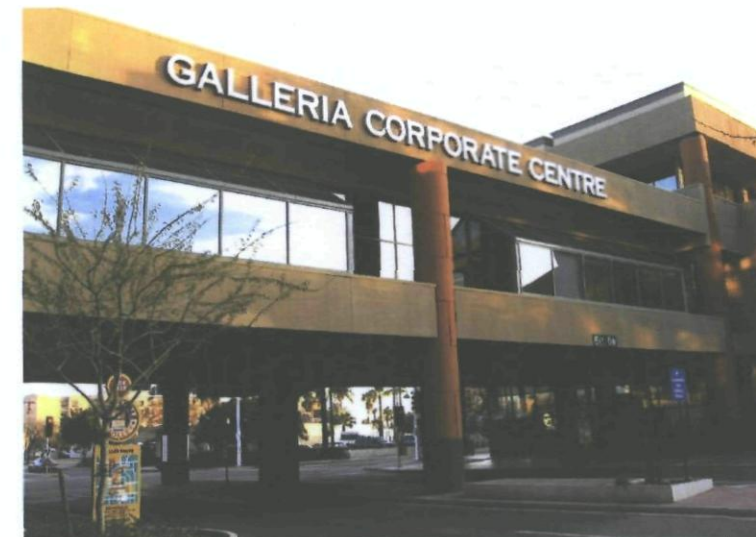
Halo illuminated reverse pan-channel letter examples.
