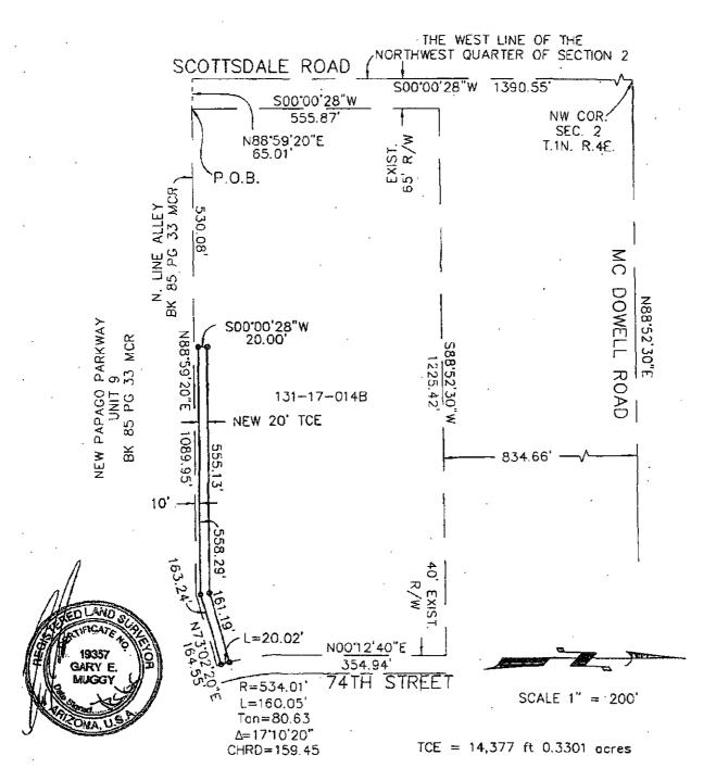
A.P.N. 131-17-014 B TEMPORARY CONSTRUCTION EASEMENT
