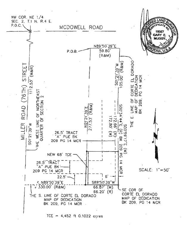
A.P.N. 131-12-080 C TEMPORARY CONSTRUCTION EASEMENT EXHIBIT-B-1
