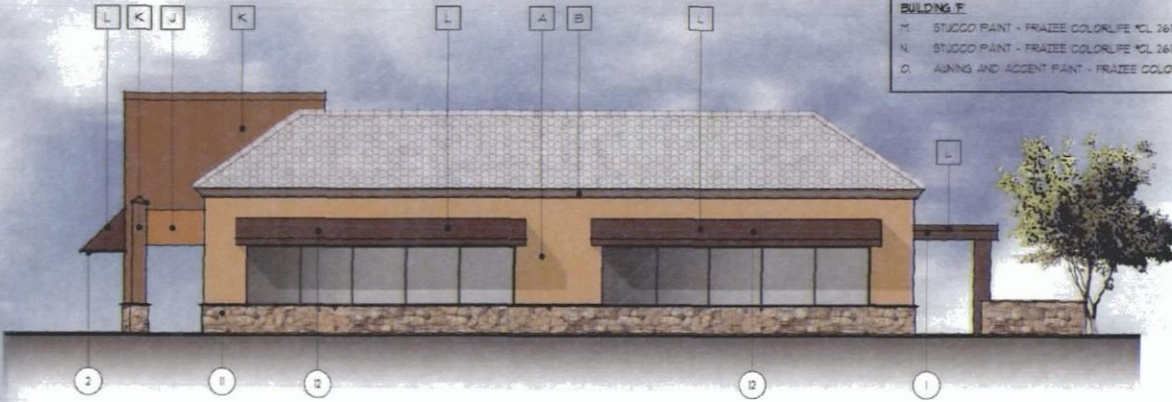
BUILDING E NORTH RENOVATED ELEVATION 2 SCALE: 1/8" = 1'-0"
