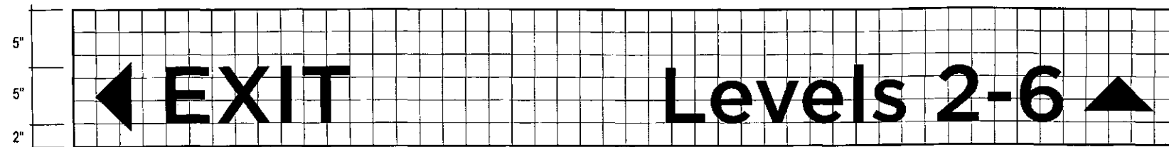
4 SIGN TYPE G3: LAYOUT 2" GRID 1"=1'-0"
