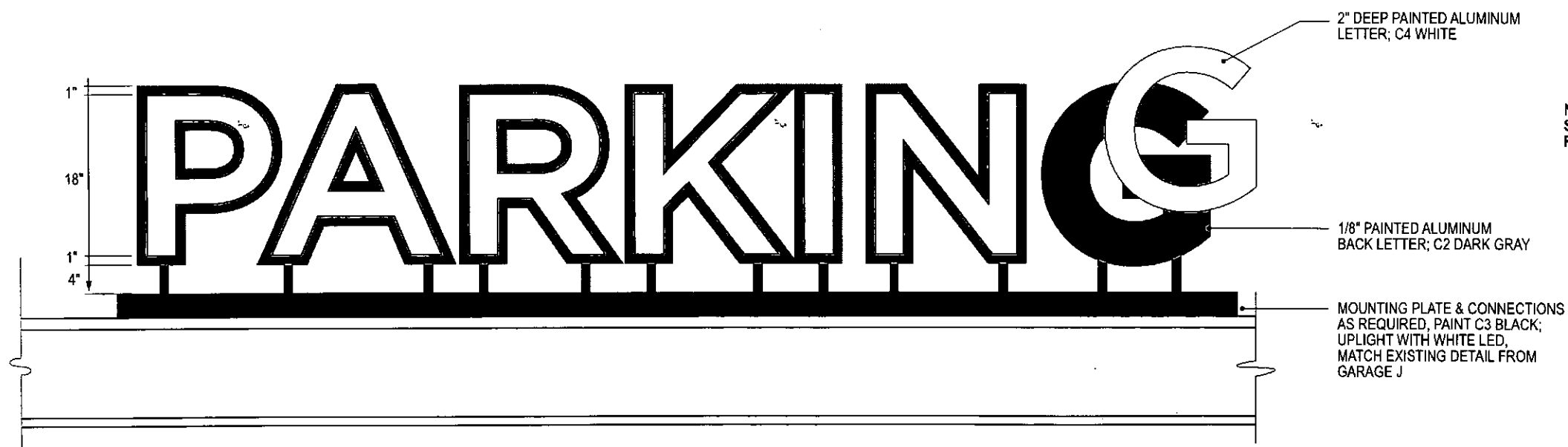
1 SIGN TYPE G1: DESIGN INTENT ELEVATION 3/4"=1'-0"
