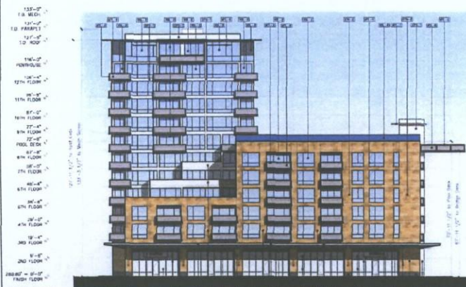
WEST ELEVATION Note: Transparent (window) area at this elevation = 65%
