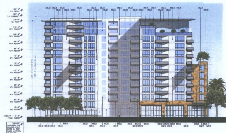
NORTH ELEVATION Note: Transparent (window) area at this elevation = 57%
