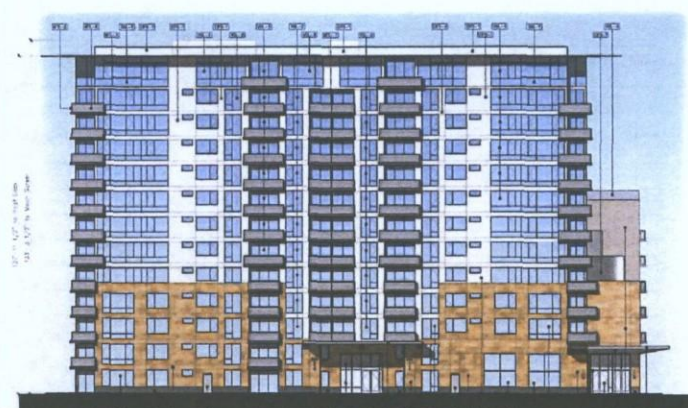
NORTH ELEVATION Note: Transparent (window) area at this elevation = 57%
