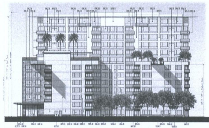
SOUTH ELEVATION Note: Transparent (window) area at this elevation = 55%
