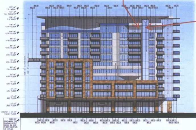
WEST ELEVATION Note: Transparent (window) area at this elevation = 68%
