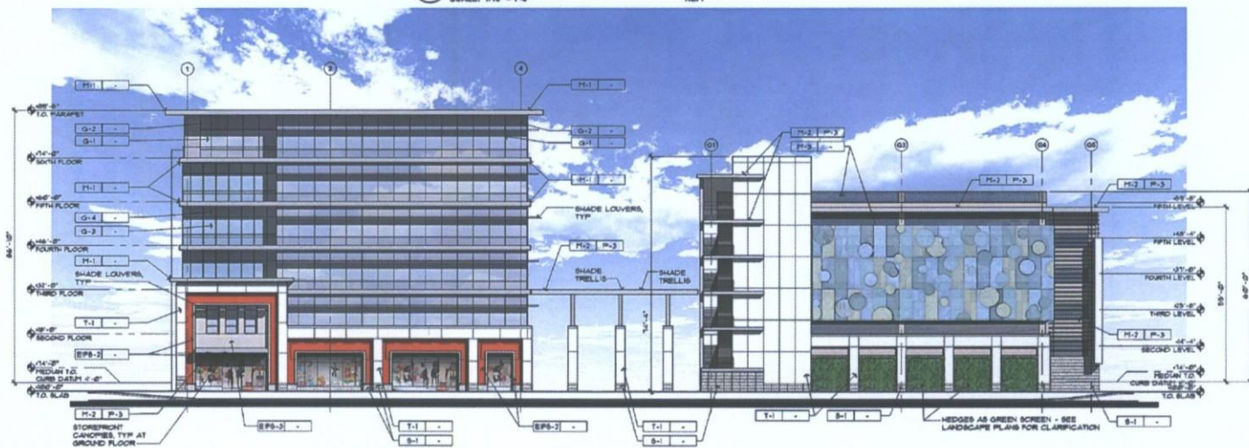
02 NORTH ELEVATION SCALE: 1/16" = 1'-0"
