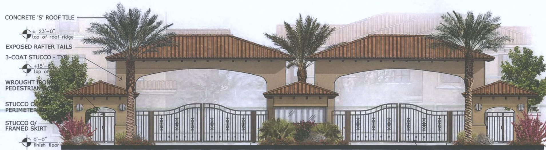
FRONT ELEVATION - PORTE COCHERE
