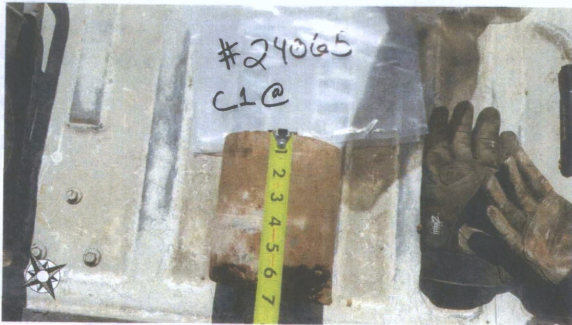
Core 1 thickness is variable; with the average being 6.0 inches.
