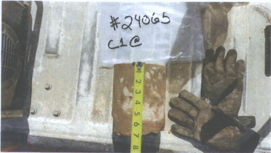
Core 1 thickness in this image is an average of 6.0 inches. One edge extends to 7.0 inches, but that is not the typical thickness.
