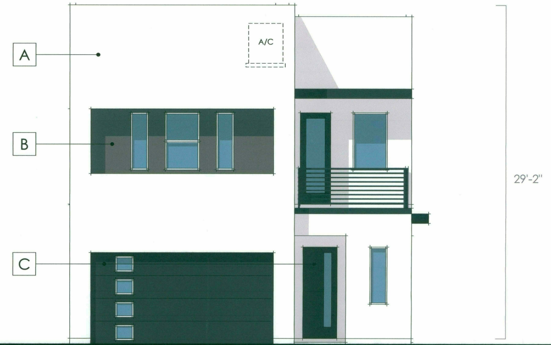
FRONT ELEVATION AT RIGHT EXPOSED CORNER
