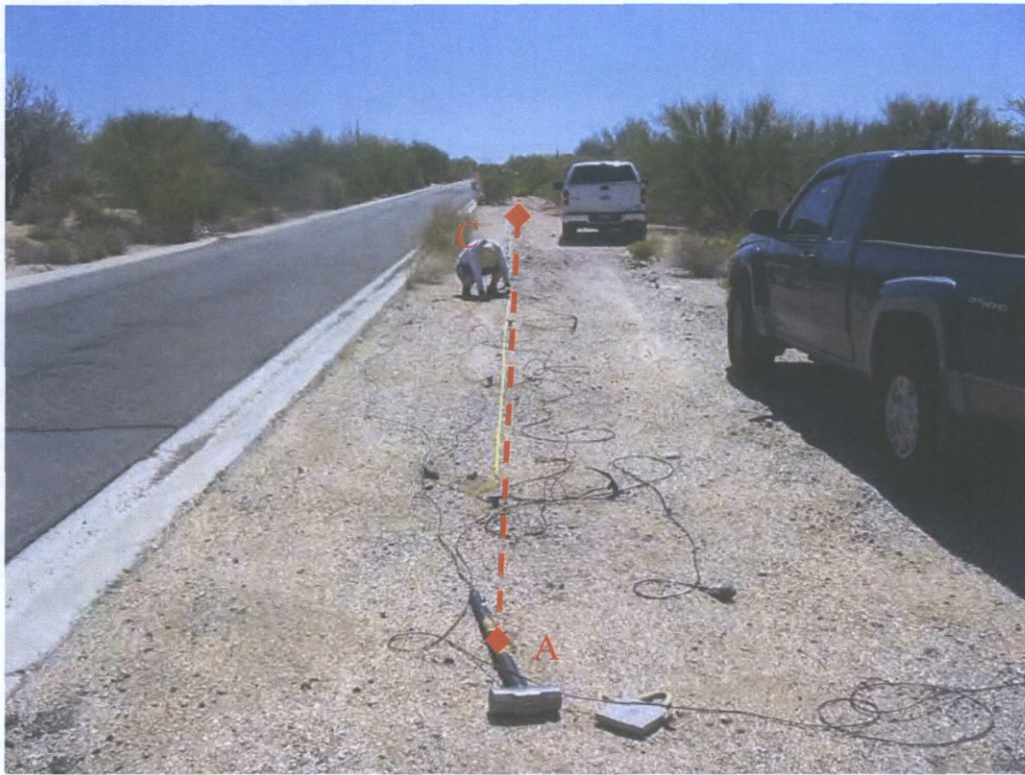
Figure 4; Photo 1: Seismic Survey Line BM-S1 view looking toward the east from Shot Point A toward Shot Point C.
