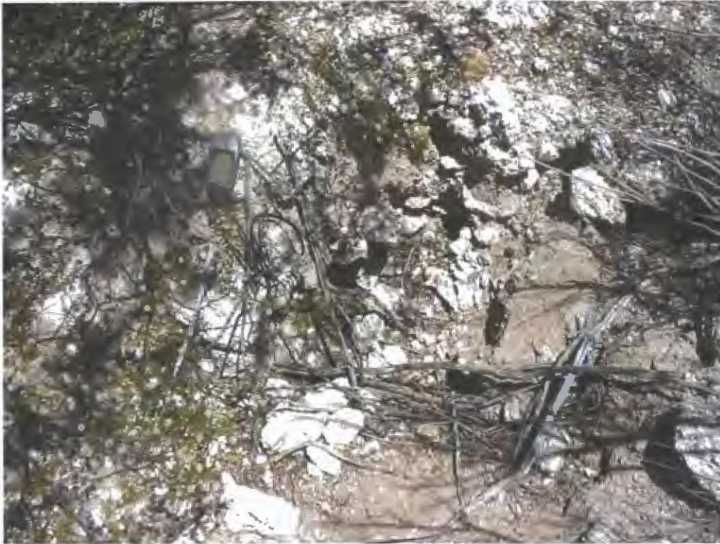
Figure 21; Photo 1: Portion of caliche cemented overburden soil formed above the contact boundary separating the overburden soil from the underlying granite bedrock. Exposure in shallow stream channel cut near the east end of seismic line BM-S3.
