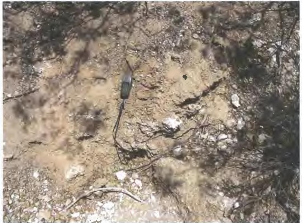
Figure 21; Photo 2: Close-up view of tan to light brown, weathered, caliche-cemented overburden cap. Exposure in shallow stream channel cut near the east end of seismic line BM-S3.
