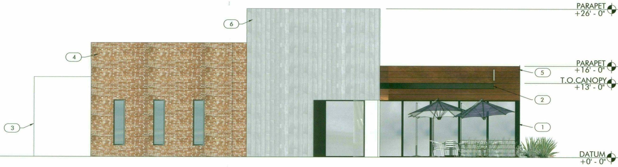
7 CONCEPTUAL SOUTH ELEVATION - BUILDING B SCALE: 1/8" = 1'-0"
