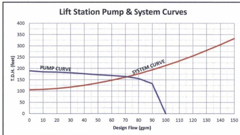
Approximate Capacity at C = 130: 71 gpm
