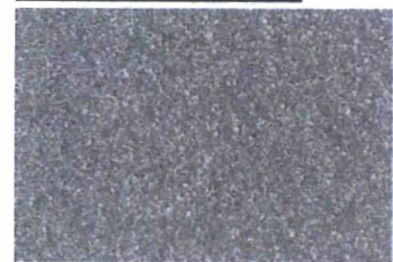
Acid Etched Concrete
