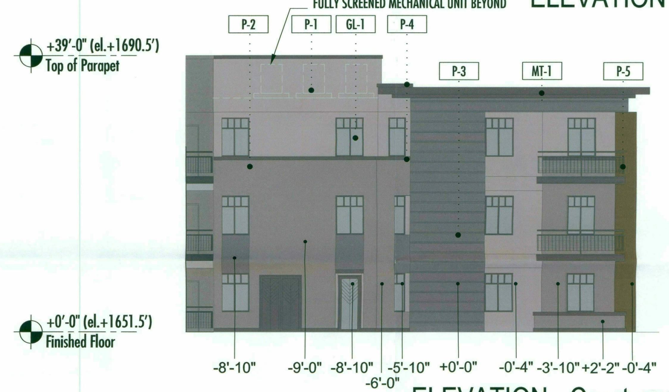
ELEVATION - Courtyard South
