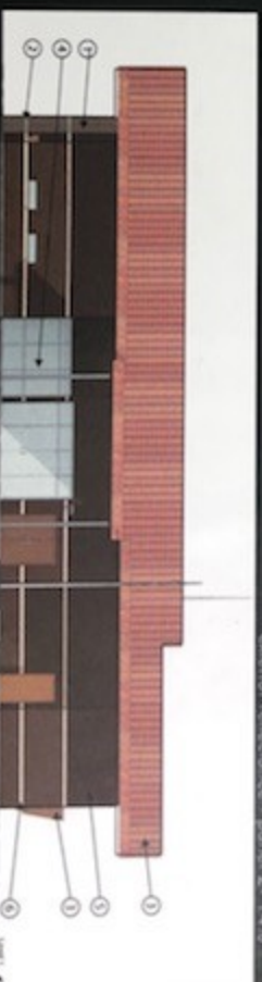
4 SOLARCOOL - SOLARBRONZE glass exterior reflectance - panel 1: 37% exterior reflectance - panel 2: 14%
