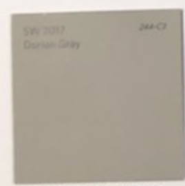
EFIS-2: 1" EFIS SYSTEM, SAND FINISH COLOR: SW 7017 "DORIAN GRAY"
