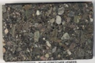
CMU-1: TRENDSTONE - 8"x18" STRETCHER VENEER, STACKED BOND COLOR: "BLACK CANYON"
