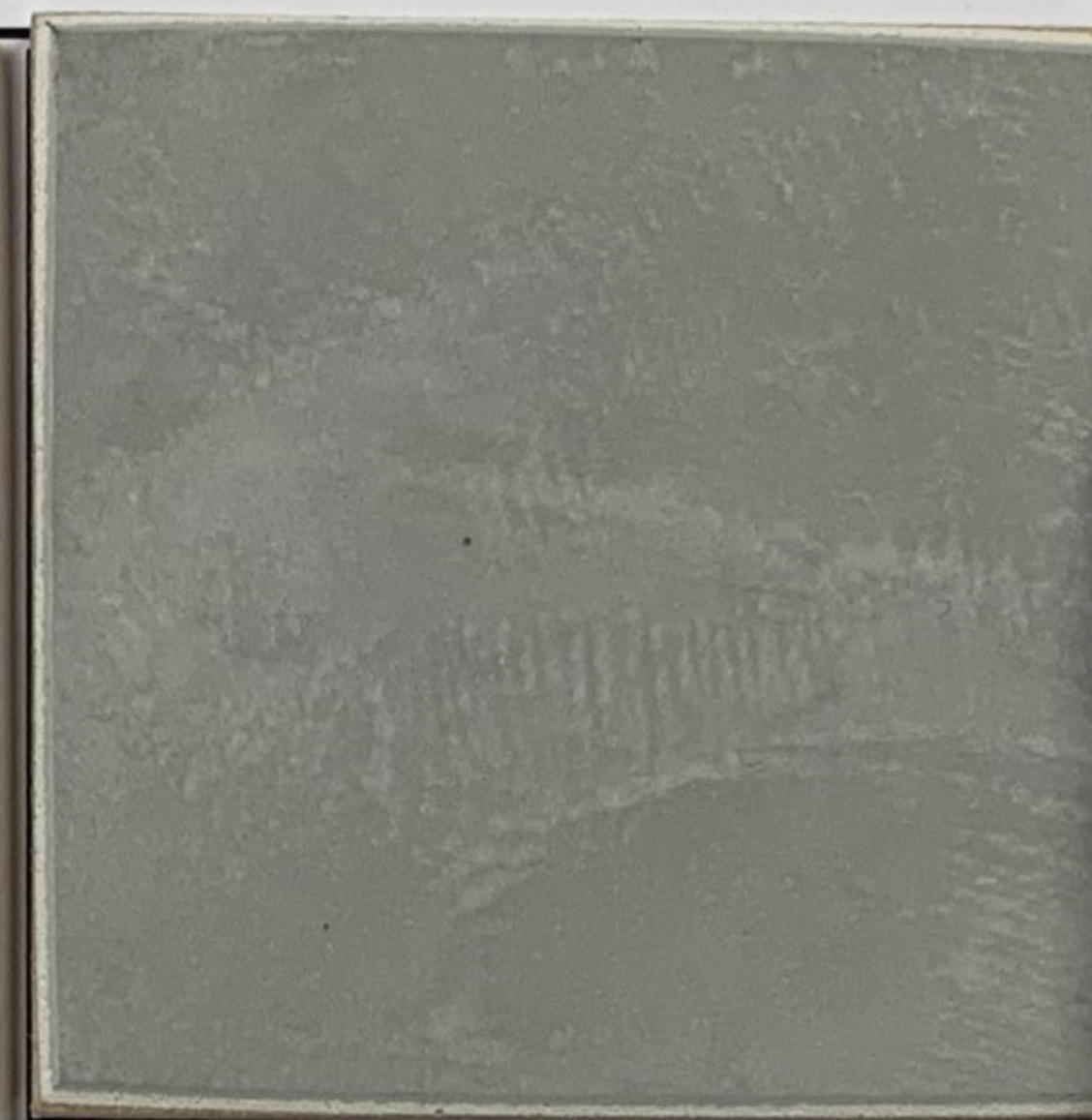
stc-2 integral color stucco - smooth finish w/ parex 'plateau' '3019L (50)'
