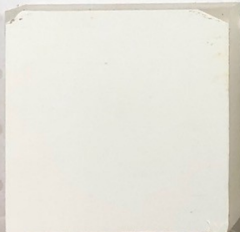
3/4" clear acrylic with 3m #230-20 translucent white vinyl overlays on the faces with 3m White diffuser overlays for the backs.
