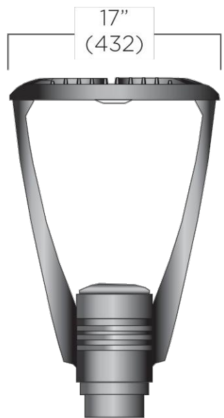
MA20 Luminaire less shade. EPA: 0.93
