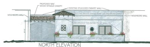
NORTH ELEVATION PROPOSED FRONT ELEVATION
