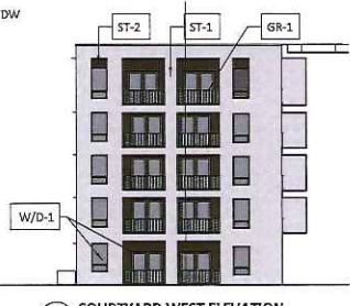
2 COURTYARD WEST ELEVATION A.1.1 1/16" = 1'-0"
