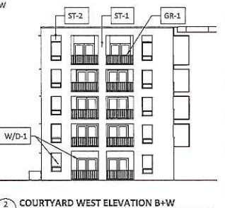
2 COURTYARD WEST ELEVATION B+W 1/16" = 1'-0"
