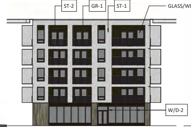
3 COURTYARD SOUTH ELEVATION A.1.1 1/16" = 1'-0"
