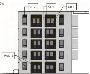
2 COURTYARD WEST ELEVATION A.1.1 1/16" = 1'-0"
