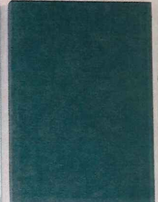
GL01S PRODUCT: SPANDEL GLASS MANUFACTURER: VIRACON FINISH: 1/4" PACIFIC-27 WITH V948 MEDIUM GREY FRIT ON #2 SURFACE
