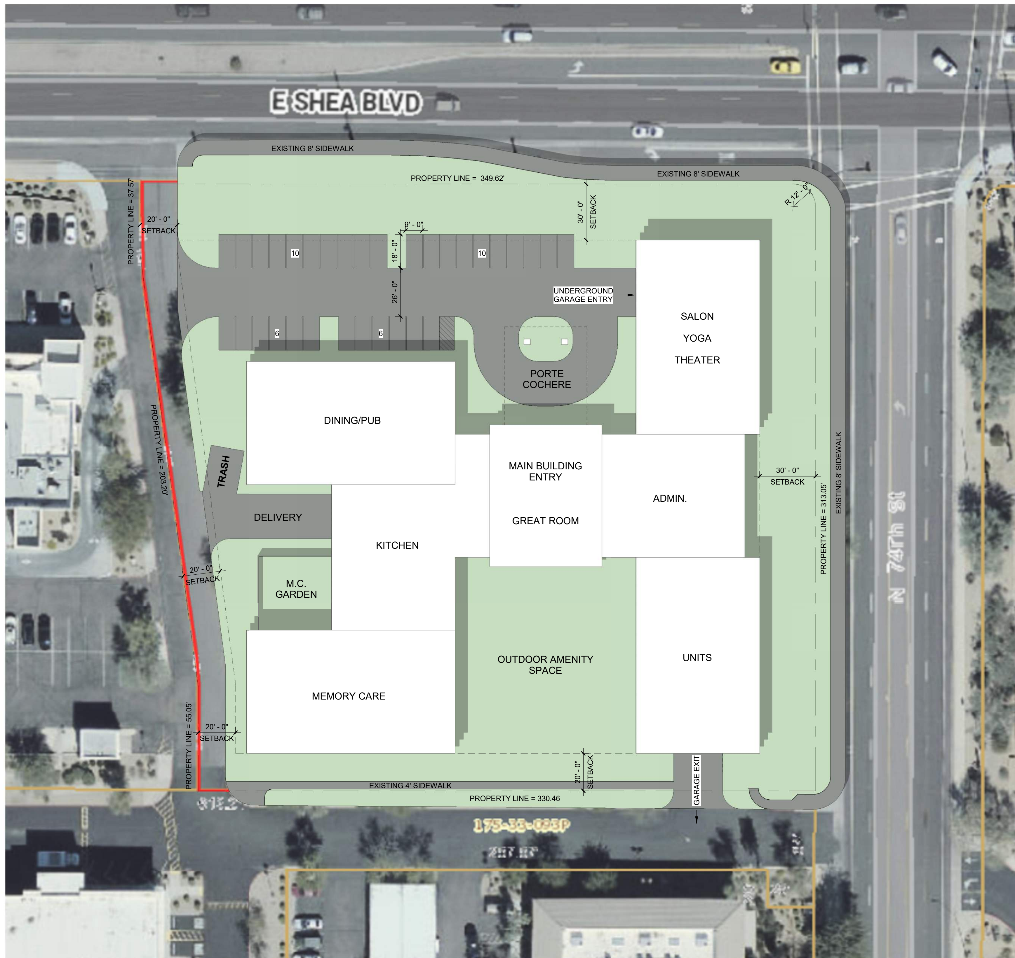
1 PROPOSED SITE PLAN A050 1" = 30'-0"
