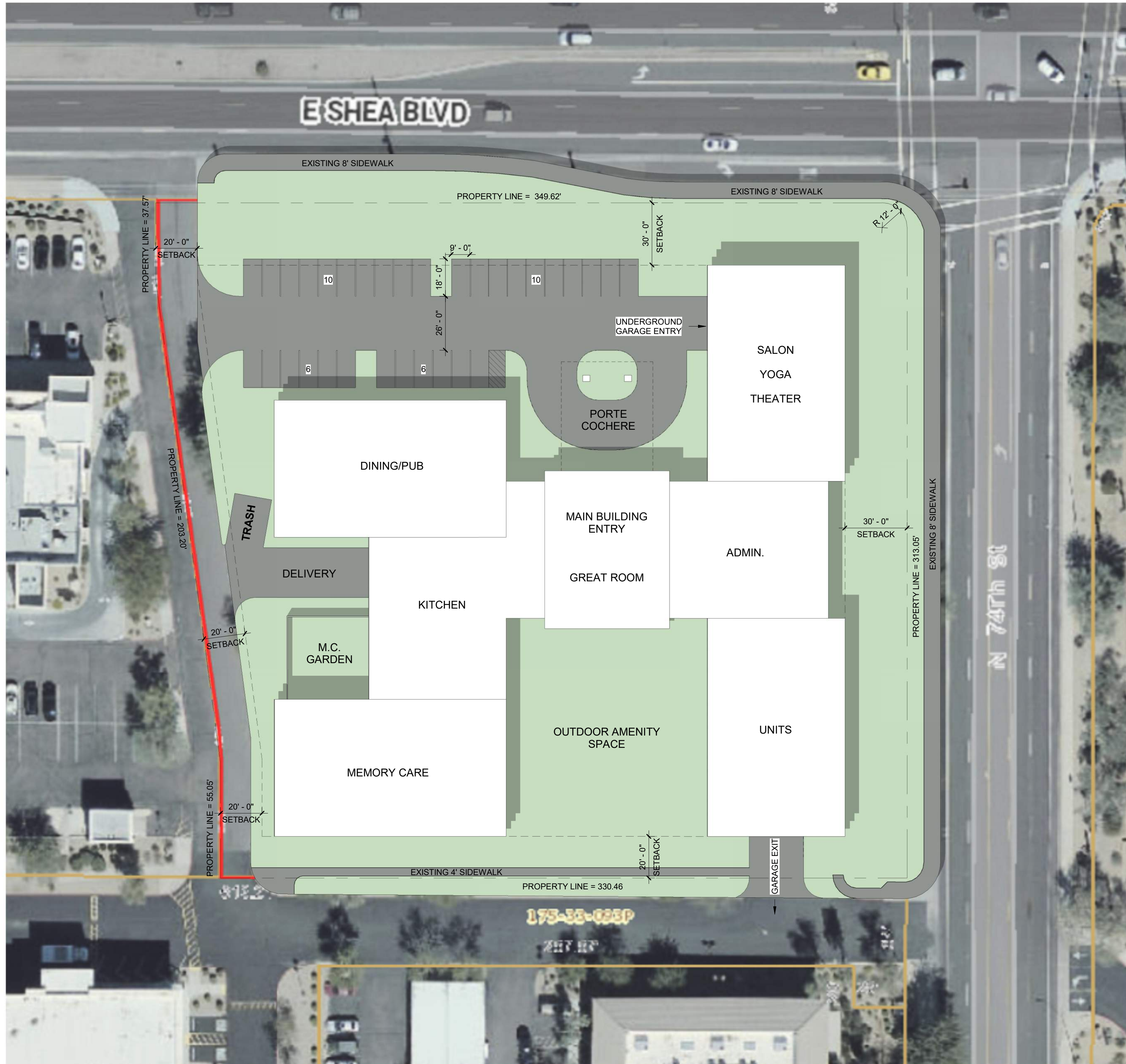
1 PROPOSED SITE PLAN A050 1" = 30'-0"
