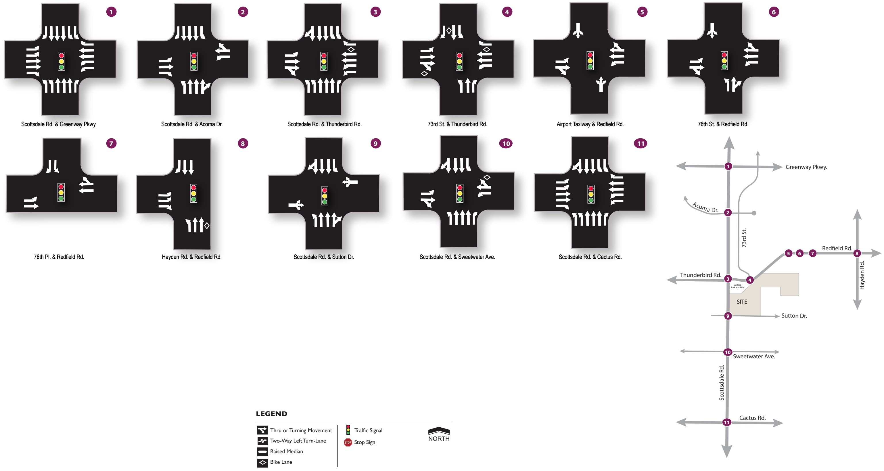
Figure 2: Existing Lane Configurations and Traffic Controls
