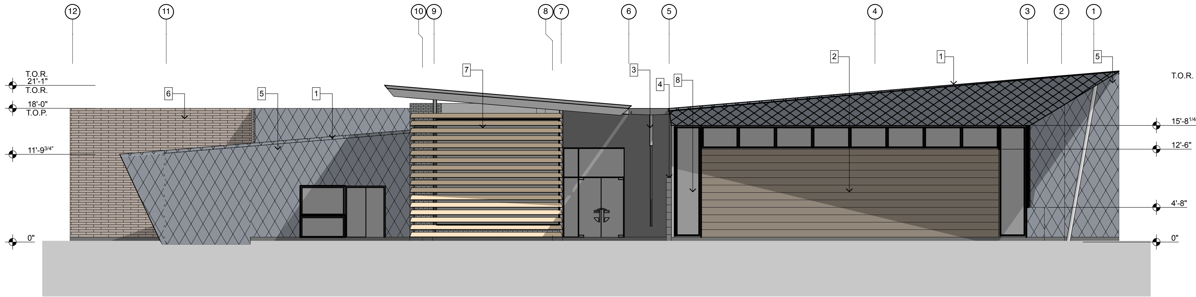
2 EAST ELEVATION SCALE: 1/8" = 1'-0" 0 4' 8' 16'
