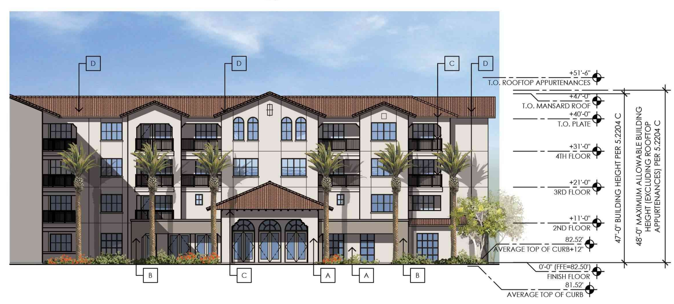
3 WEST COURTYARD ELEVATION SCALE: 1/16" = 1'-0"
