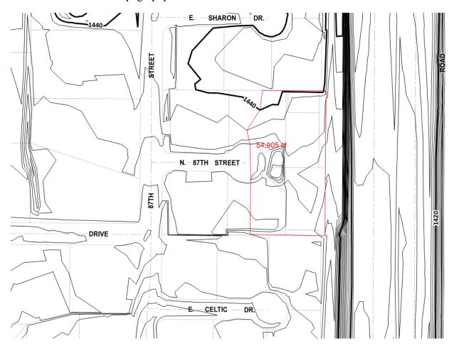
Total drainage area is approximately 54.905 square feet. The 100-year 2-hour rainfall depth is 2.24" based on the NOAA-14 precipitation table.
