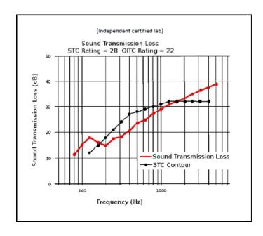
**Sound Transmission Loss Test Results**
