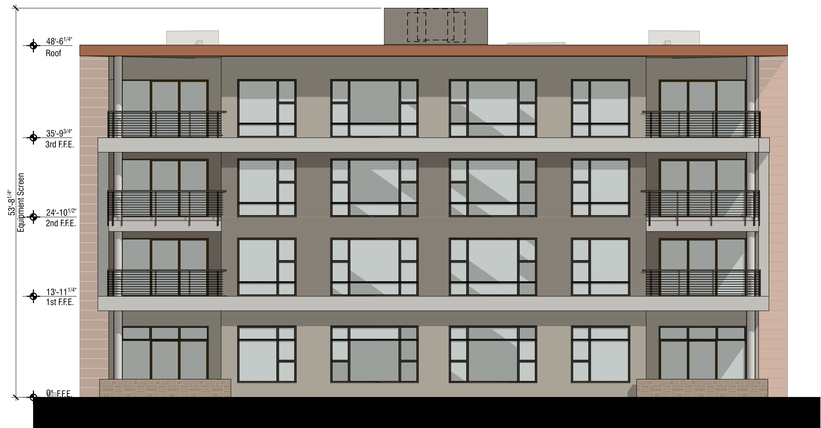
B Minimal Care South Wing - East Elevation 0 4' 8' 16' SCALE: 1/8" = 1'-0"
