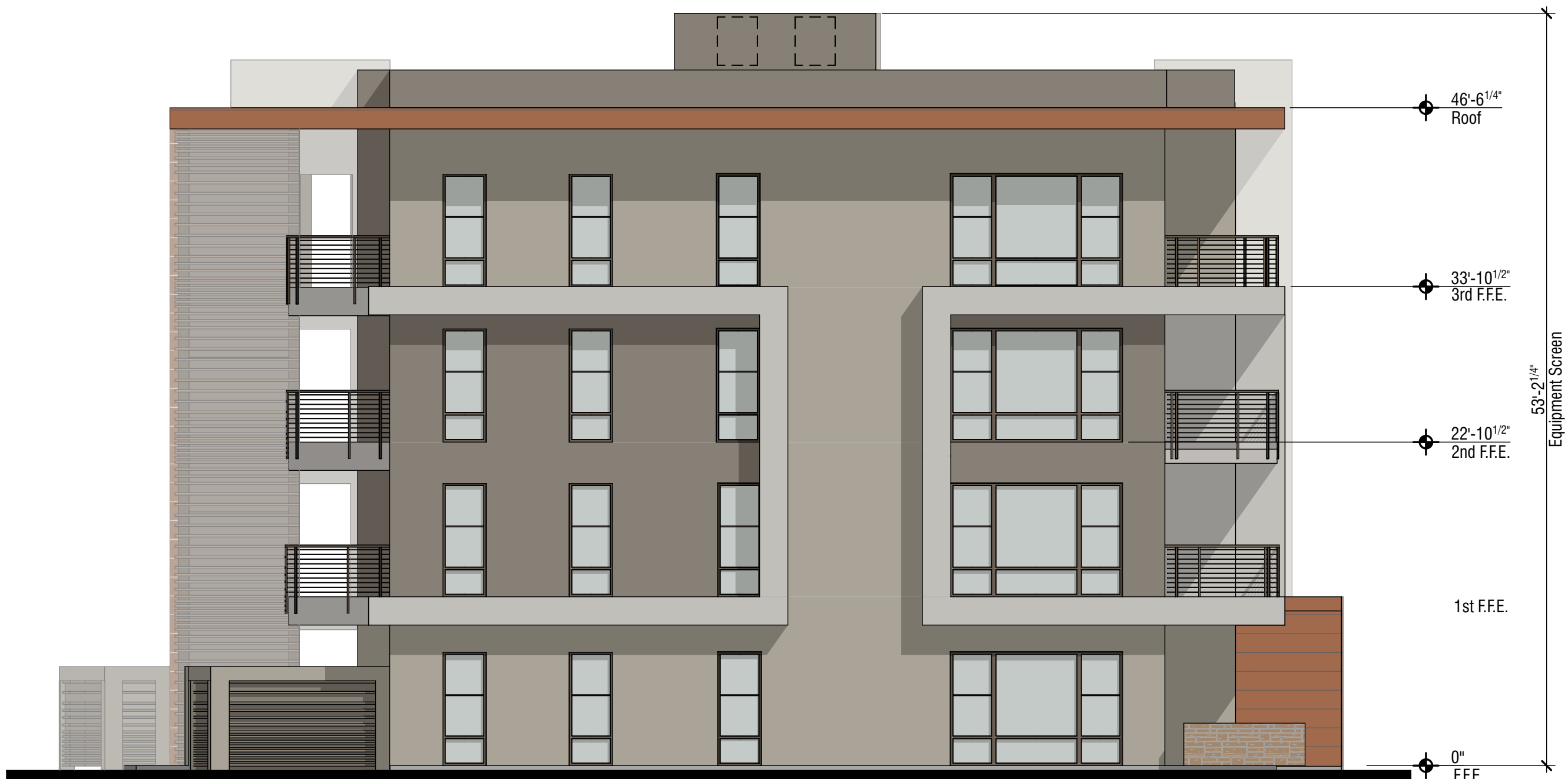
B Minimal Care North Villa - West Elevation 0 4' 8' 16' SCALE: 1/8" = 1'-0"
