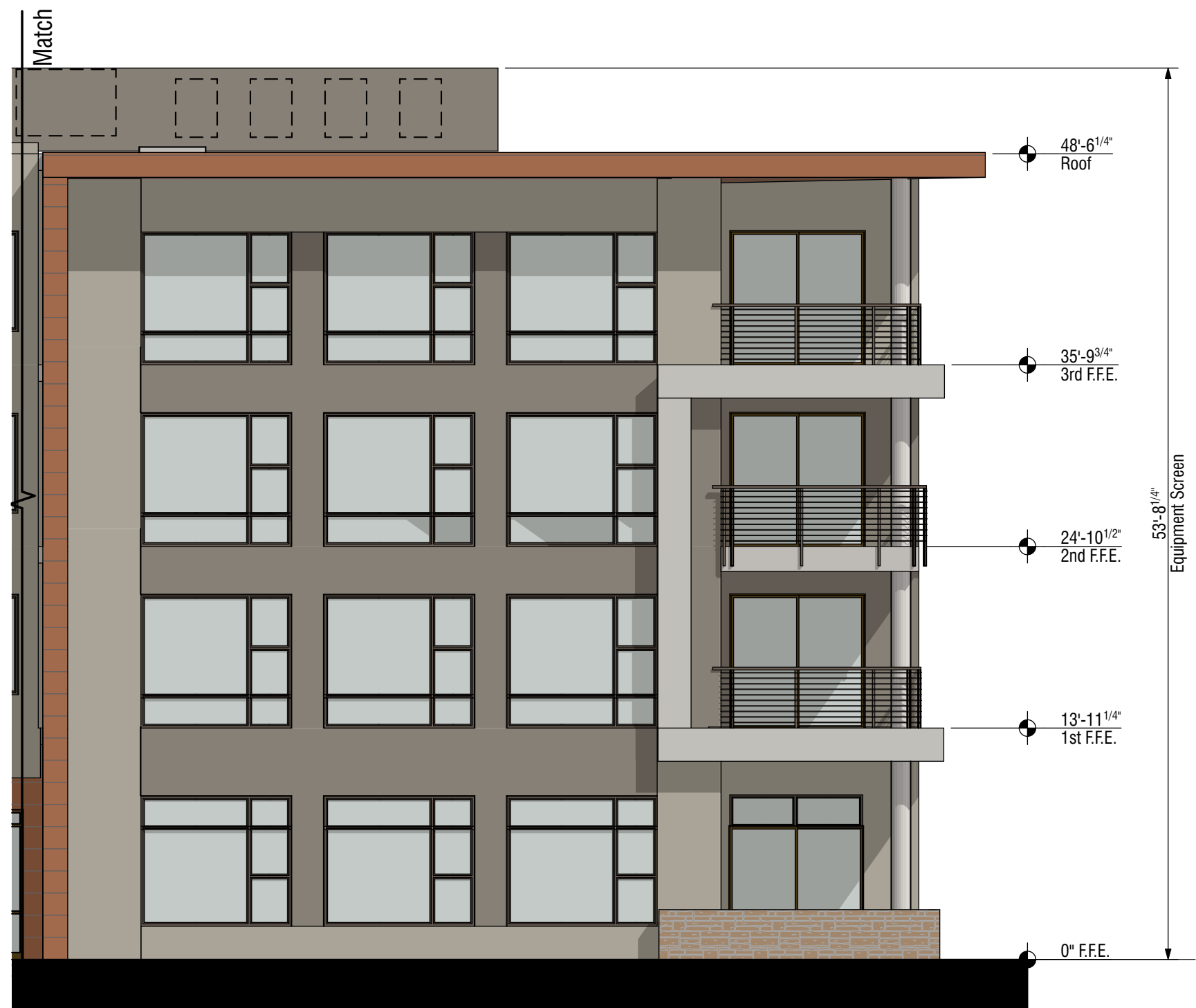
B Minimal Care East Courtyard - North Elevation 0 4' 8' 16' SCALE: 1/8" = 1'-0"
