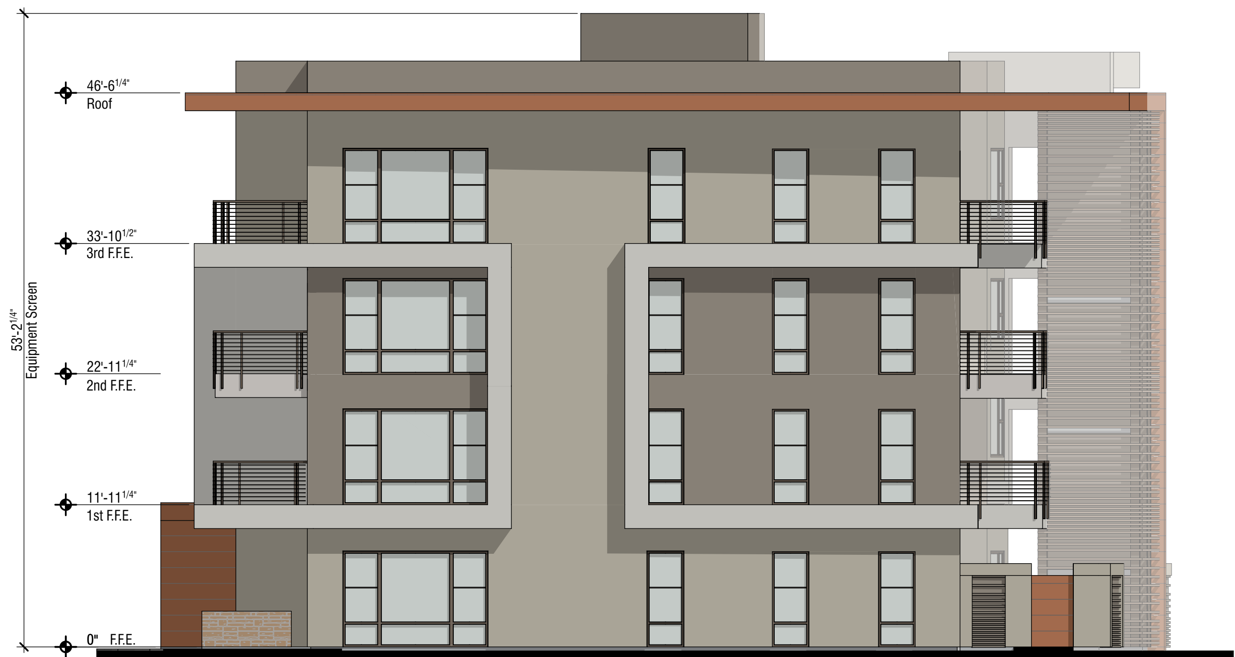
B Minimal Care South Villa - West Elevation 0 4' 8' 16' SCALE: 1/8" = 1'-0"
