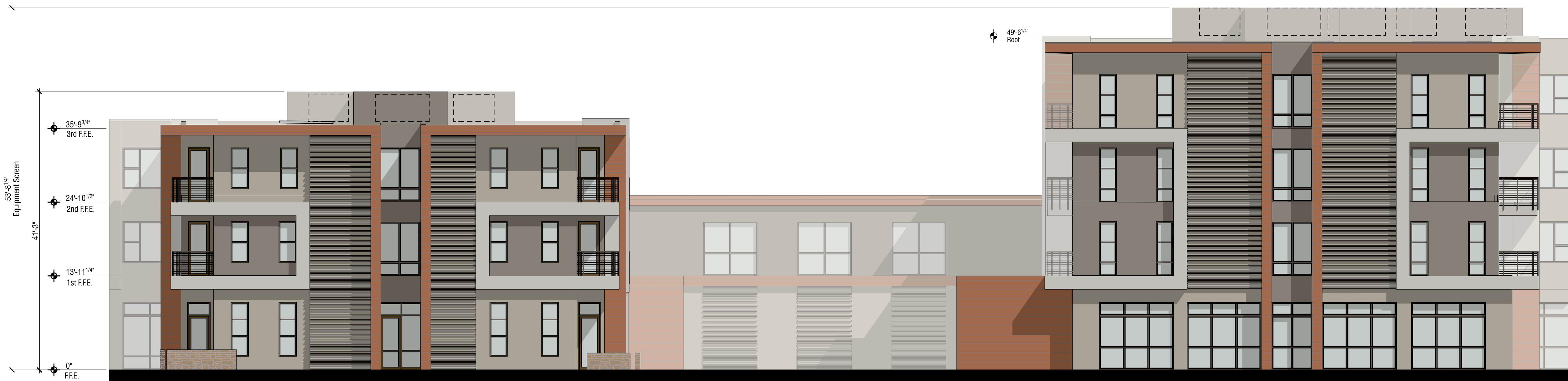
A Specialized Care/Personal Southeast Wing - South Elevation 0 4' 8' 16' SCALE: 1/8" = 1'-0"
