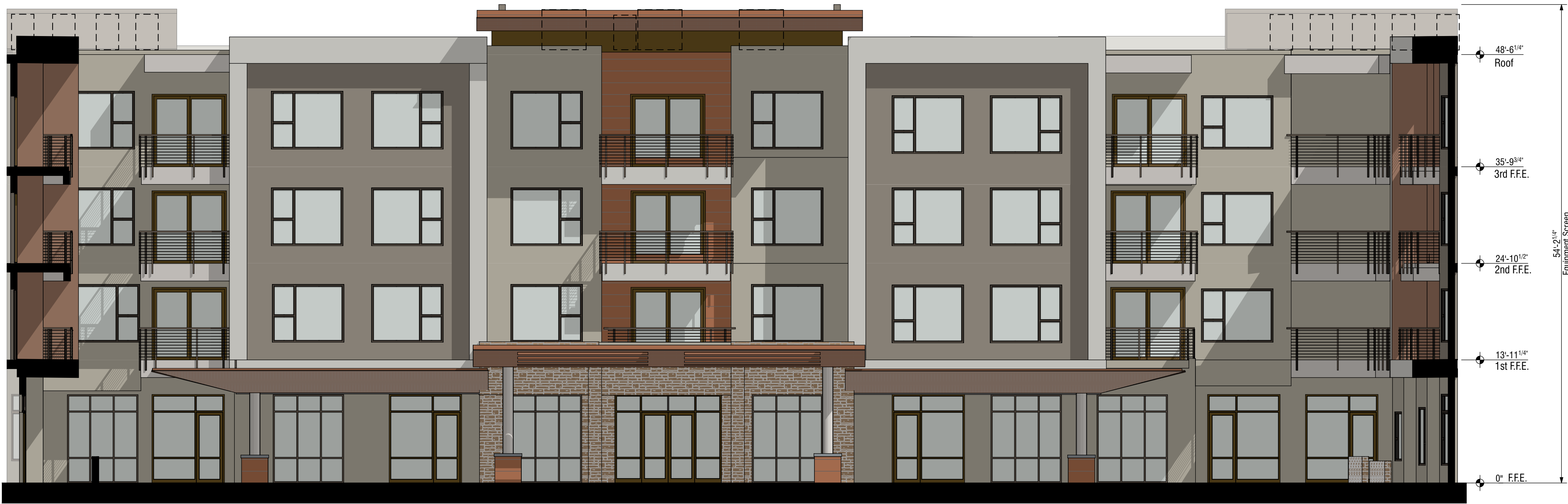
C Minimal Care East Courtyard - West Elevation 0 4' 8' 16' SCALE: 1/8" = 1'-0"
