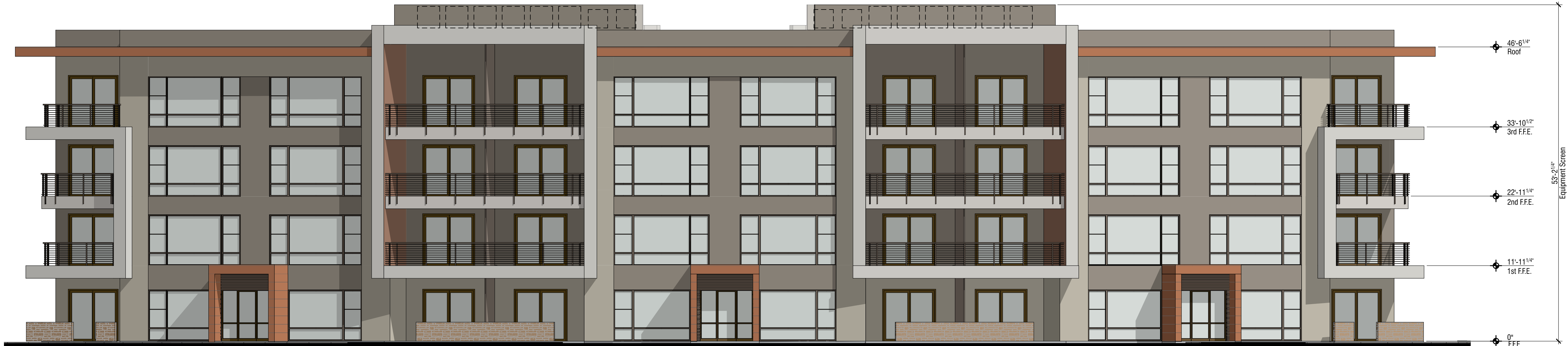
A Minimal Care South Villa - North Elevation 0 4' 8' 16' SCALE: 1/8" = 1'-0"
