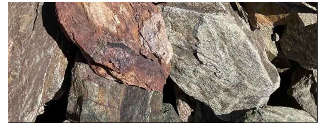
(6) '1-10' DESERT PAVEMENT: SUPPLIER: ROCK PROS USA COLOR: 3-6" RIP RAP, ASH
