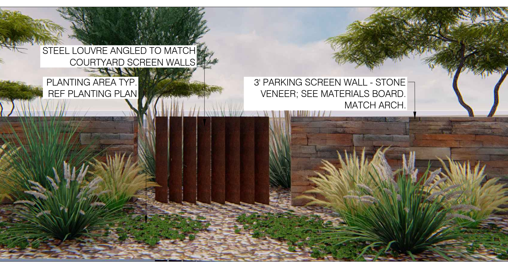
8 3' PARKING SCREEN WALL (ELEVATION) NTS
