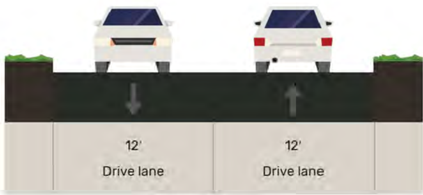
SECTION B1-a 2 LANES - NO PARKING NTS
