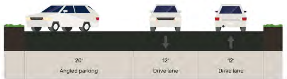
SECTION B6 2 LANES - 60° PARKING ON ONE SIDE NTS
