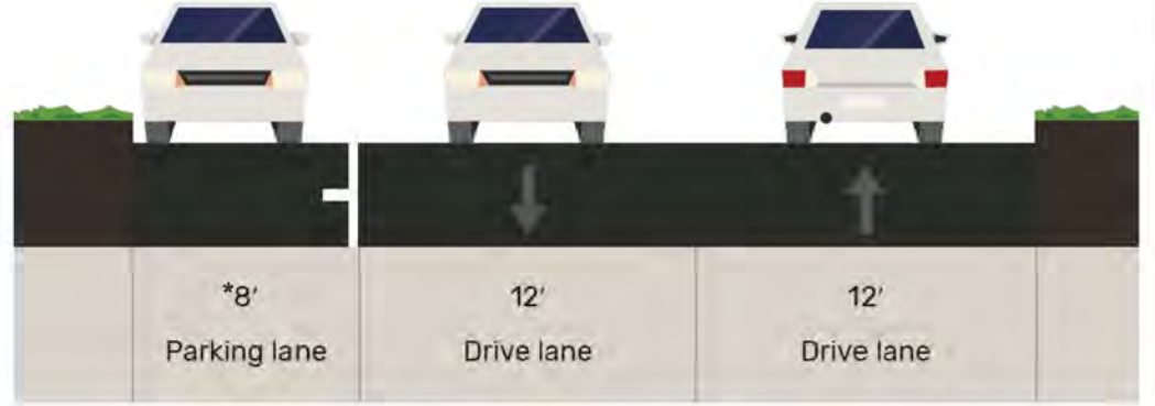
SECTION B5-a 2 LANES - PARALLEL PARKING ON ONE SIDE NTS *8 TO 9 FEET WIDTH AS APPROVED BY CITY STAFF
