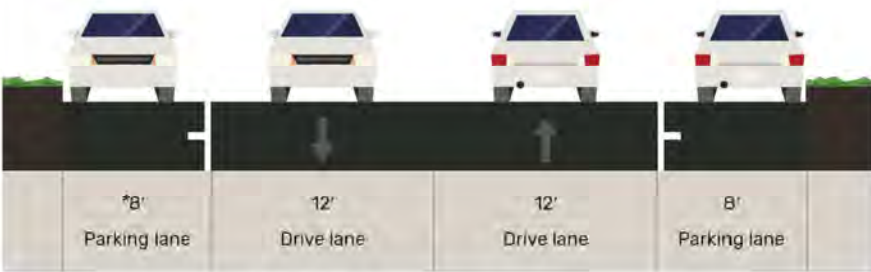
SECTION B2-a 2 LANES - PARALLEL PARKING ON BOTH SIDES NTS * 8 TO 9 FEET WIDTH AS APPROVED BY CITY STAFF
