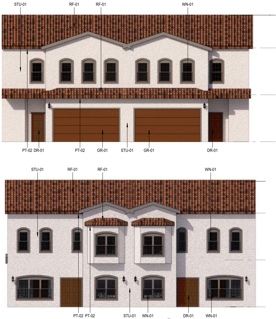
PLANNING AREA 2 - TYPICAL ELEVATIONS
