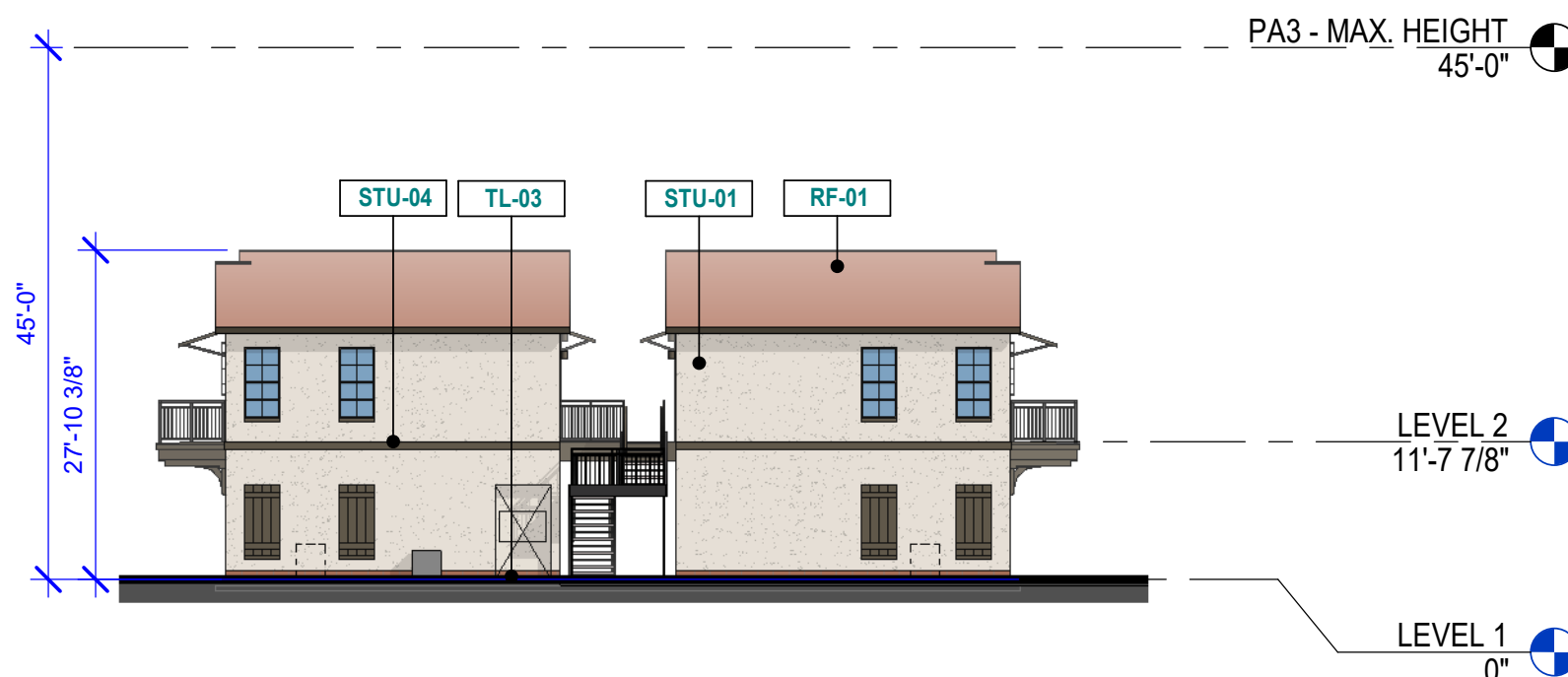
01 TYPICAL TREEHOUSE - BACK ELEVATION 1/16" = 1'-0"
