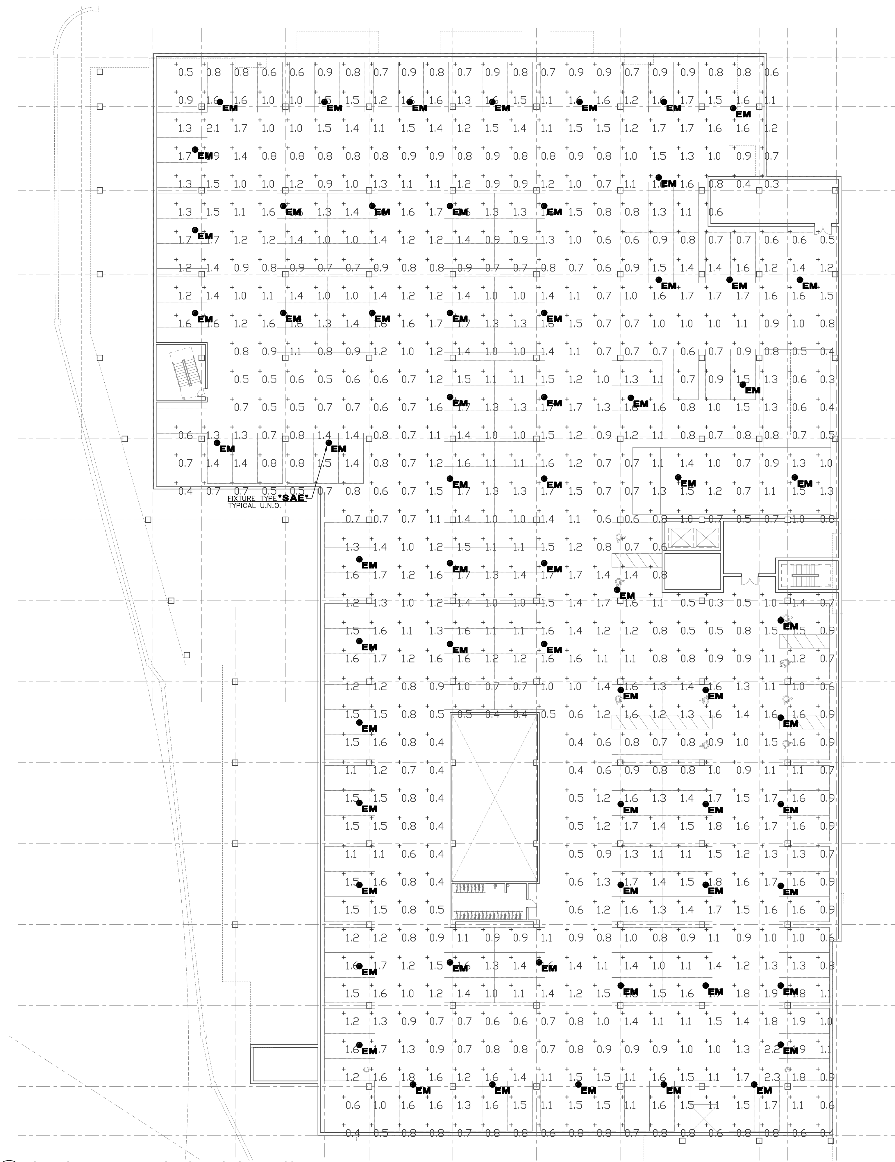
1 GARAGE LEVEL 1 EMERGENCY PHOTOMETRICS PLAN DR2.3 1" = 20' - 0"
