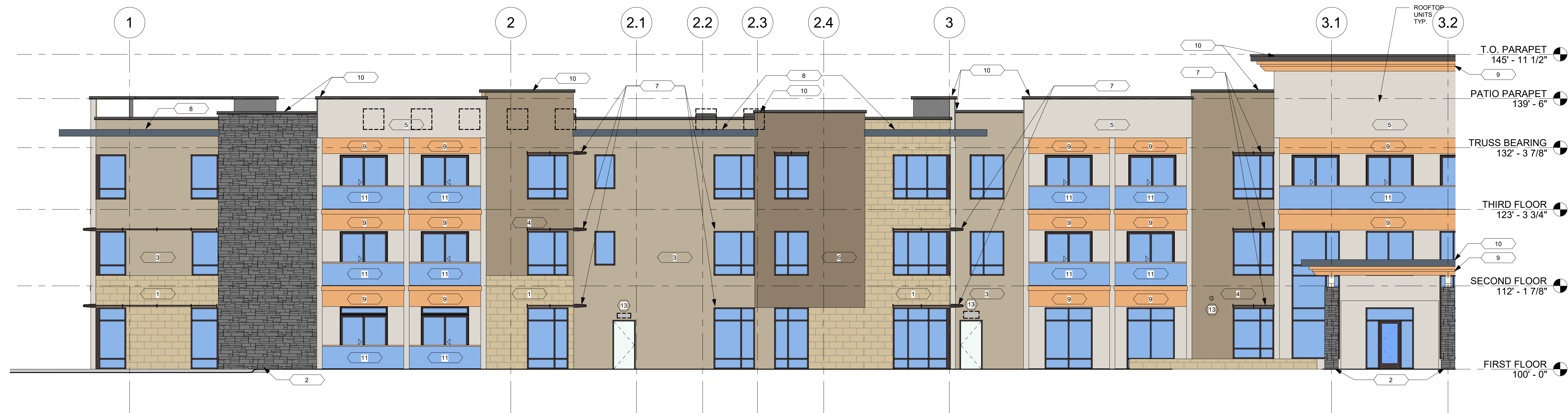
1 A300 MAIN BUILDING EXTERIOR ELEVATION "A" SCALE: 1/8" = 1'-0"
