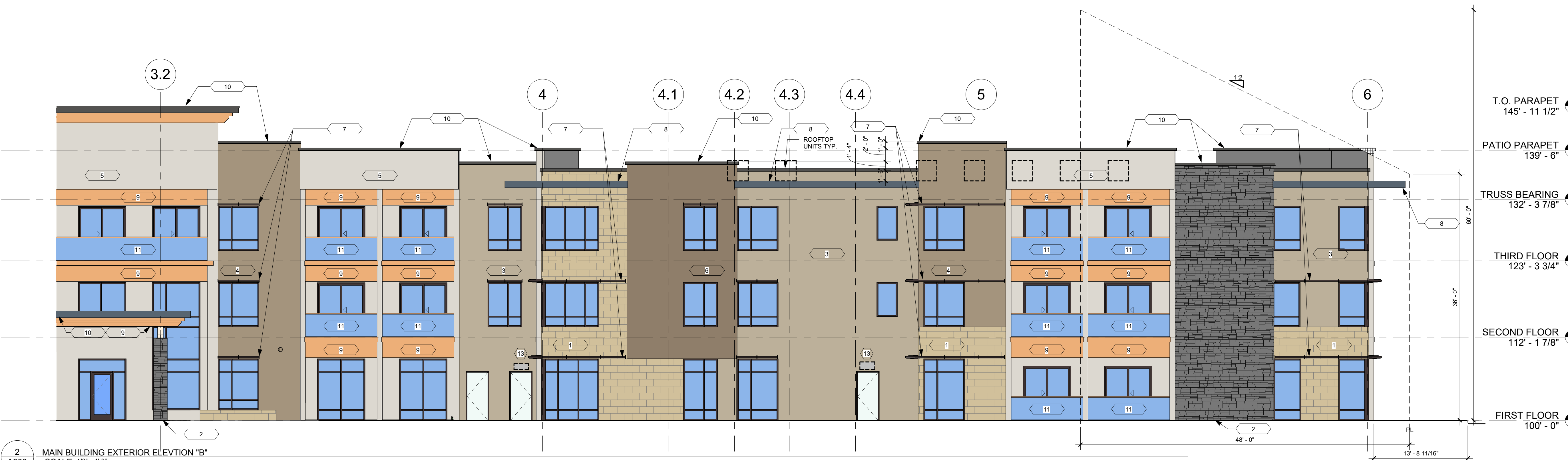
2 A300 MAIN BUILDING EXTERIOR ELEVATION "B" SCALE: 1/8" = 1'-0"
