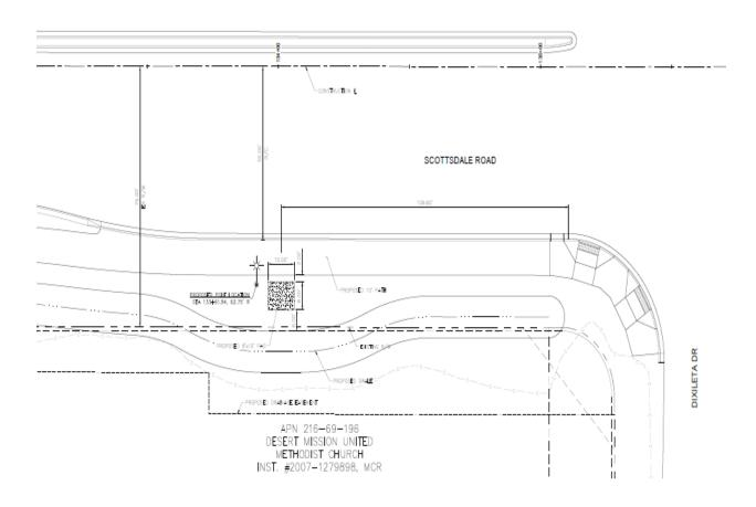
The new Dish Wireless cell site will be located in the right of way on the east side of Scottsdale Road. The antenna for the cell site will be placed on top of a new functional streetlight pole. The associated Dish equipment cabinets will also be placed in the right of way and screened from public view.
