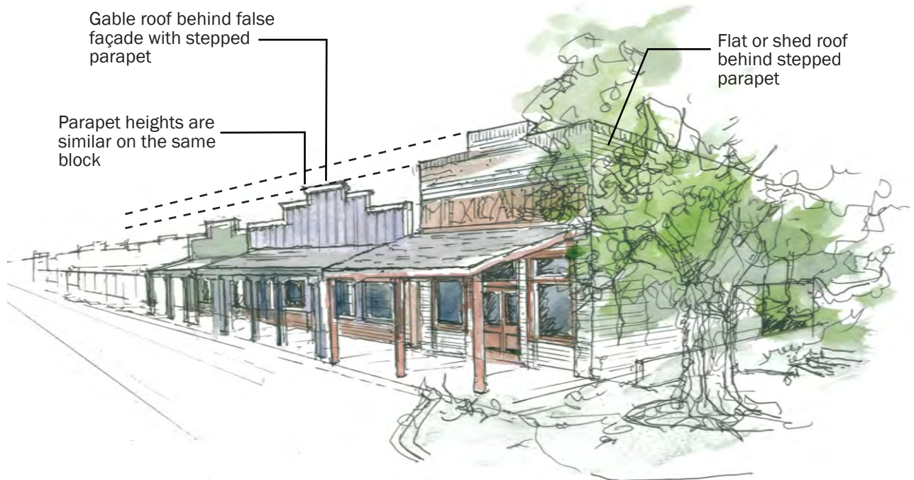
Figure 25 - Historic Old Town Architectural Design
