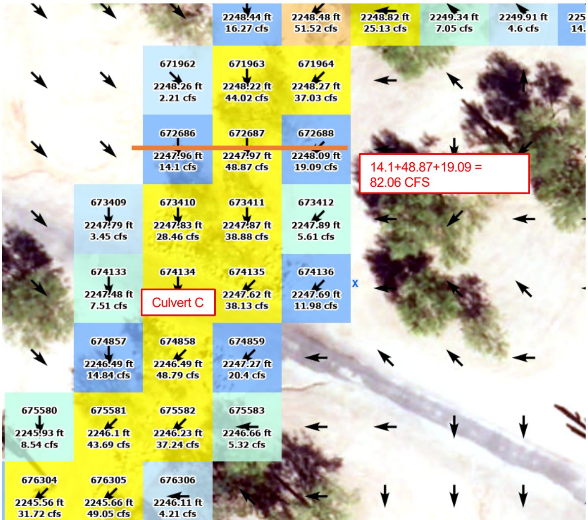
Figure 3.1.4 Flo-2D North Wash Culvert C Cross-Section Image
