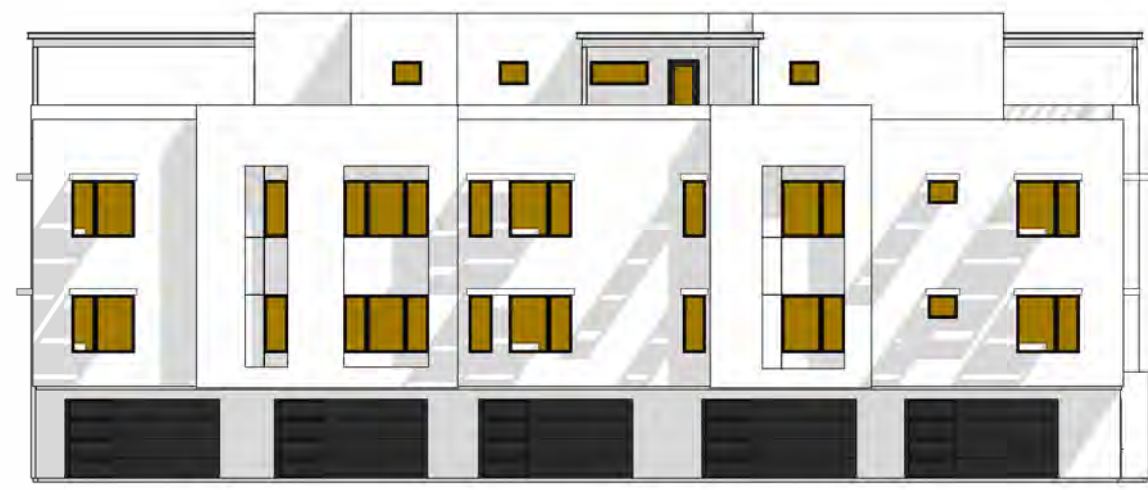
D TOTAL GLAZING: 570.1 SF SHADED GLAZING: 554.9 SF
