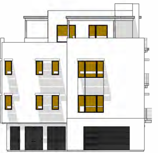
L TOTAL GLAZING: 256.7 SF SHADED GLAZING: 209.5 SF
