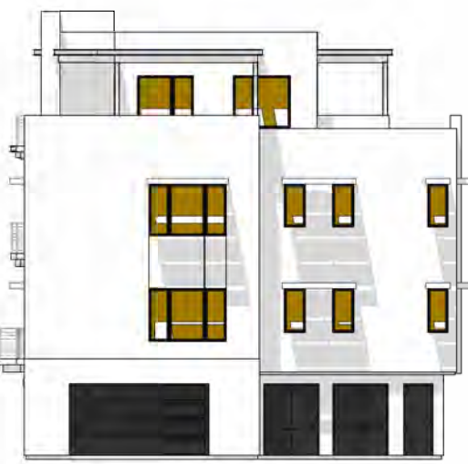
C TOTAL GLAZING: 256.7 SF SHADED GLAZING: 209.5 SF
