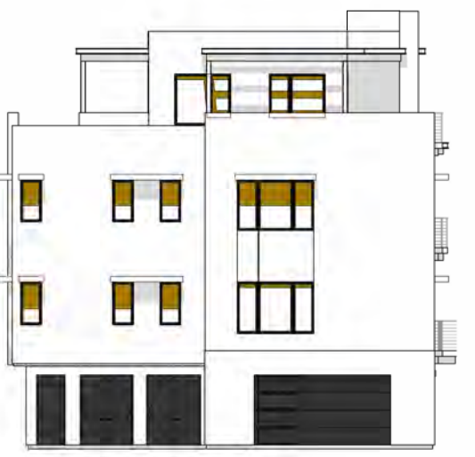
L TOTAL GLAZING: 256.7 SF SHADED GLAZING: 110.0 SF
