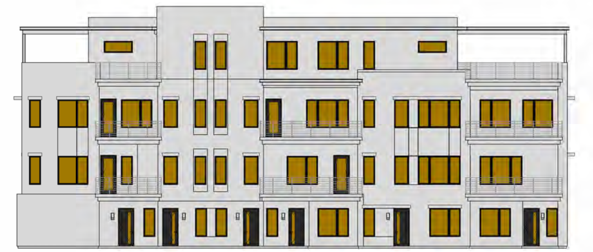
N TOTAL GLAZING: 1174.3 SF SHADED GLAZING: 1174.3 SF
