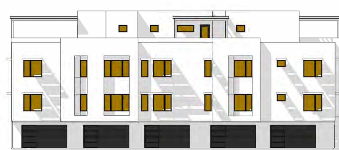
J TOTAL GLAZING: 570.1 SF SHADED GLAZING: 556.8 SF
