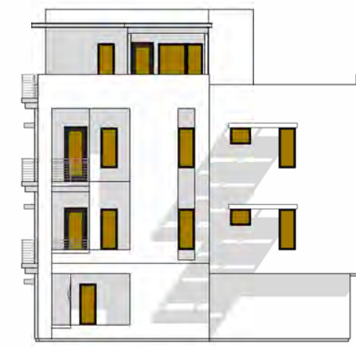
F TOTAL GLAZING: 209.5 SF SHADED GLAZING: 209.5 SF
