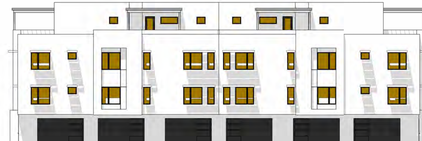
H TOTAL GLAZING: 697.7 SF SHADED GLAZING: 633.3 SF
