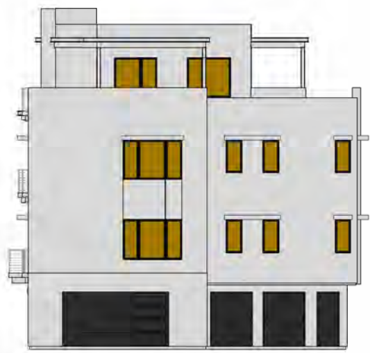
C TOTAL GLAZING: 256.7 SF SHADED GLAZING: 256.7 SF
