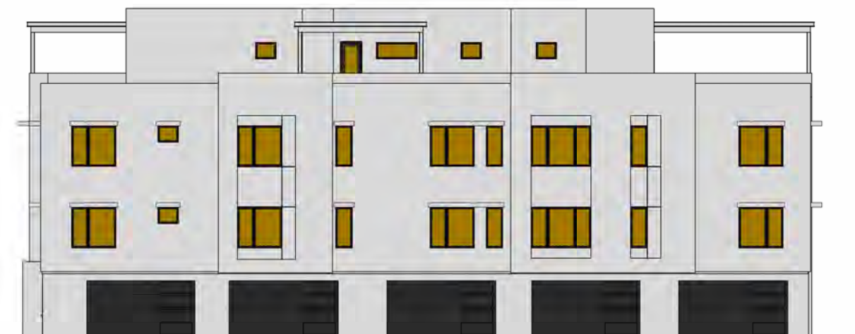
A TOTAL GLAZING: 570.1 SF SHADED GLAZING: 570.1 SF
