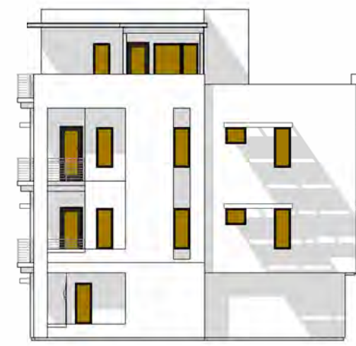
F TOTAL GLAZING: 209.5 SF SHADED GLAZING: 209.5 SF
