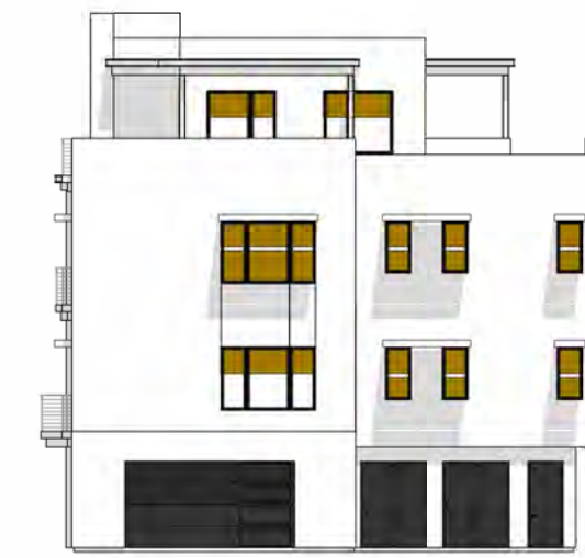
G TOTAL GLAZING: 256.7 SF SHADED GLAZING: 170.3 SF
