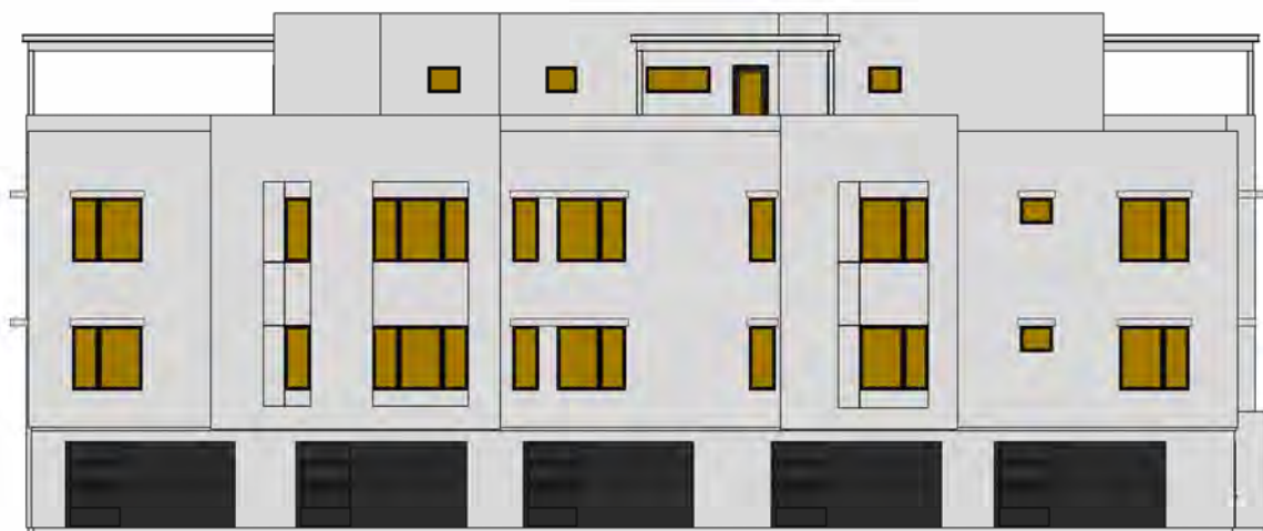
N TOTAL GLAZING: 570.1 SF SHADED GLAZING: 570.1 SF
