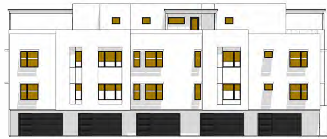
D TOTAL GLAZING: 570.1 SF SHADED GLAZING: 450.8 SF
