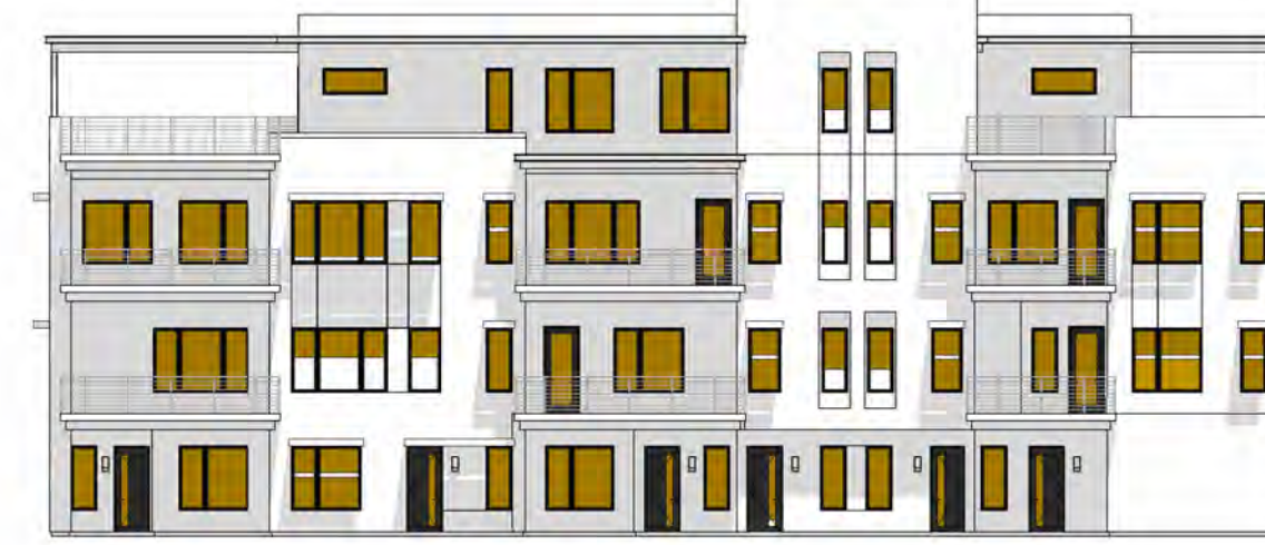
C TOTAL GLAZING: 1174.3 SF SHADED GLAZING: 1072.5 SF
