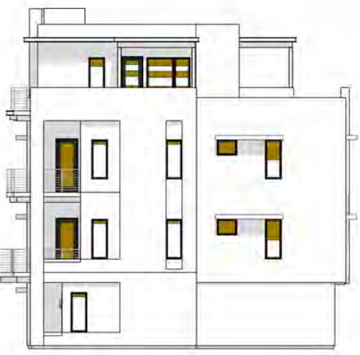
L TOTAL GLAZING: 209.5 SF SHADED GLAZING: 92.1 SF
