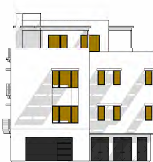
I TOTAL GLAZING: 256.7 SF SHADED GLAZING: 243.4 SF
