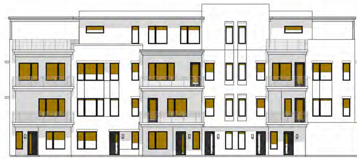
I TOTAL GLAZING: 1174.3 SF SHADED GLAZING: 686.5 SF
