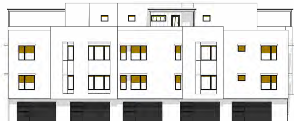
N TOTAL GLAZING: 570.1 SF SHADED GLAZING: 199.1 SF
