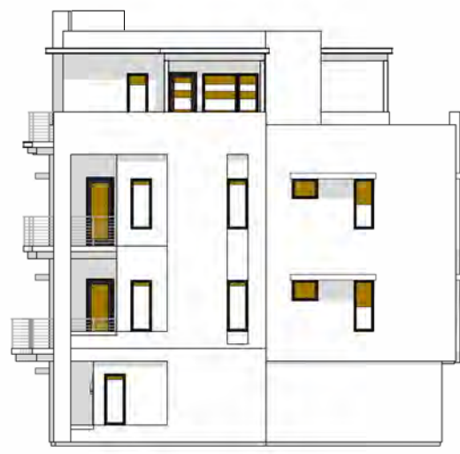
J TOTAL GLAZING: 209.5 SF SHADED GLAZING: 92.1 SF
