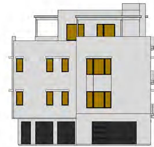
J TOTAL GLAZING: 256.7 SF SHADED GLAZING: 256.7 SF
