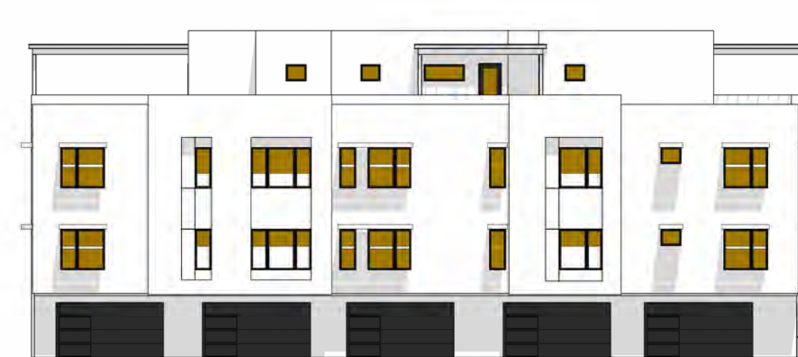
L TOTAL GLAZING: 570.1 SF SHADED GLAZING: 450.8 SF
