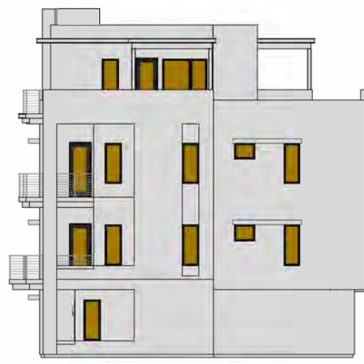
J TOTAL GLAZING: 209.5 SF SHADED GLAZING: 209.5 SF
