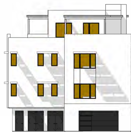
N TOTAL GLAZING: 256.7 SF SHADED GLAZING: 247.7 SF
