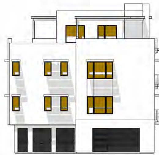
D TOTAL GLAZING: 256.7 SF SHADED GLAZING: 209.5 SF
