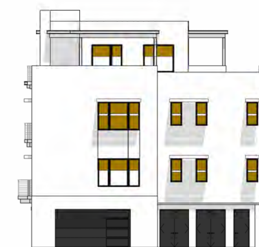
I TOTAL GLAZING: 256.7 SF SHADED GLAZING: 170.3 SF
