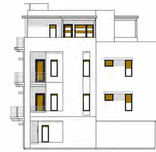
D TOTAL GLAZING: 209.5 SF SHADED GLAZING: 92.1 SF
