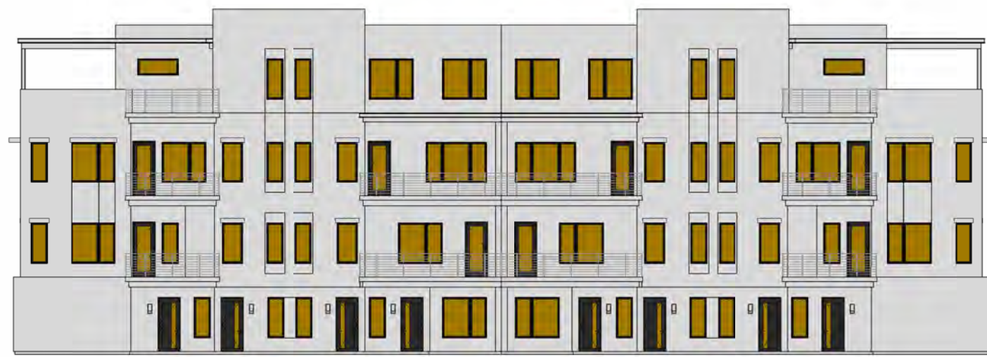
H TOTAL GLAZING: 1416.3 SF SHADED GLAZING: 1416.3 SF
