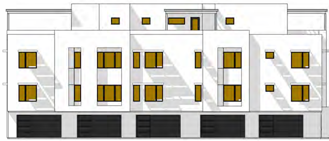
D TOTAL GLAZING: 570.1 SF SHADED GLAZING: 556.8 SF
