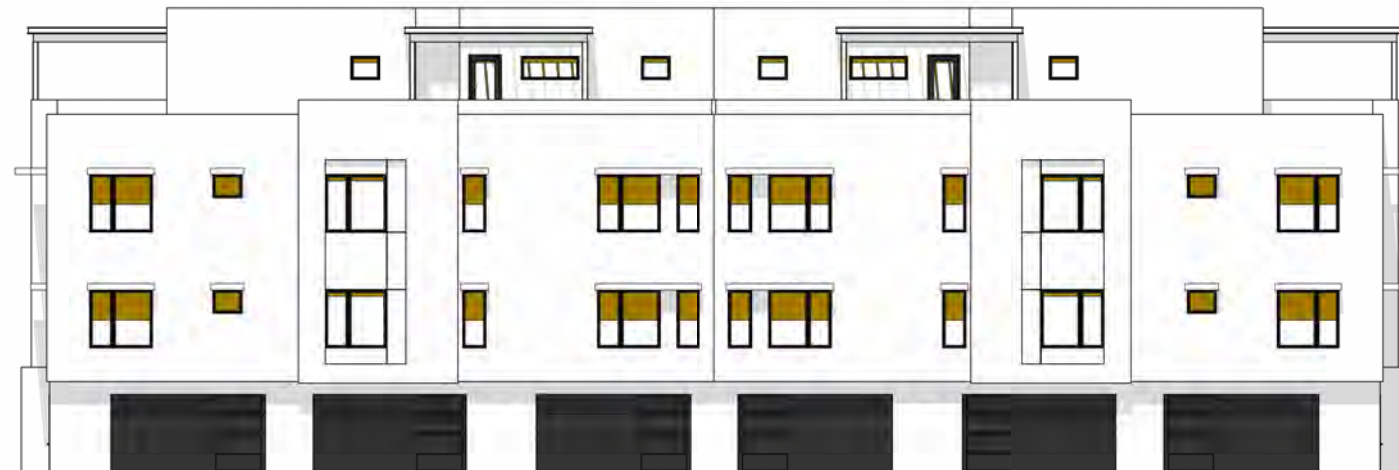
G TOTAL GLAZING: 697.7 SF SHADED GLAZING: 291.9 SF
