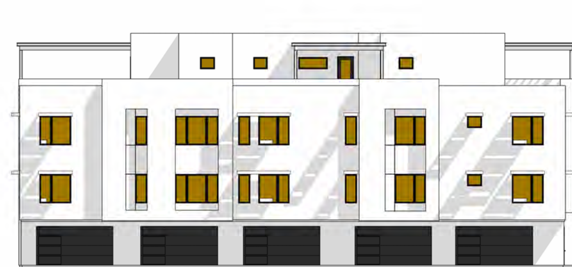
L TOTAL GLAZING: 570.1 SF SHADED GLAZING: 554.9 SF
