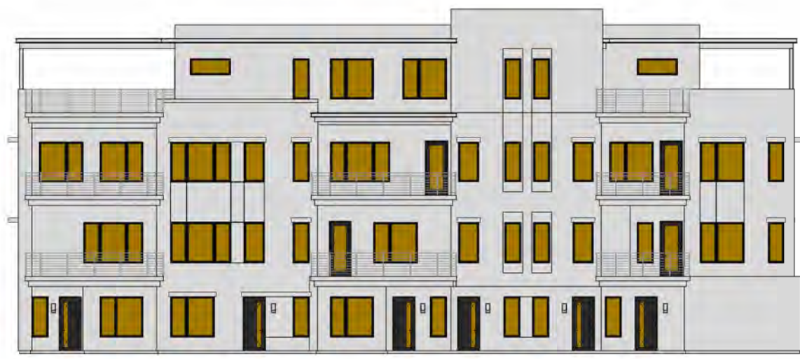
A TOTAL GLAZING: 1174.3 SF SHADED GLAZING: 1174.3 SF
