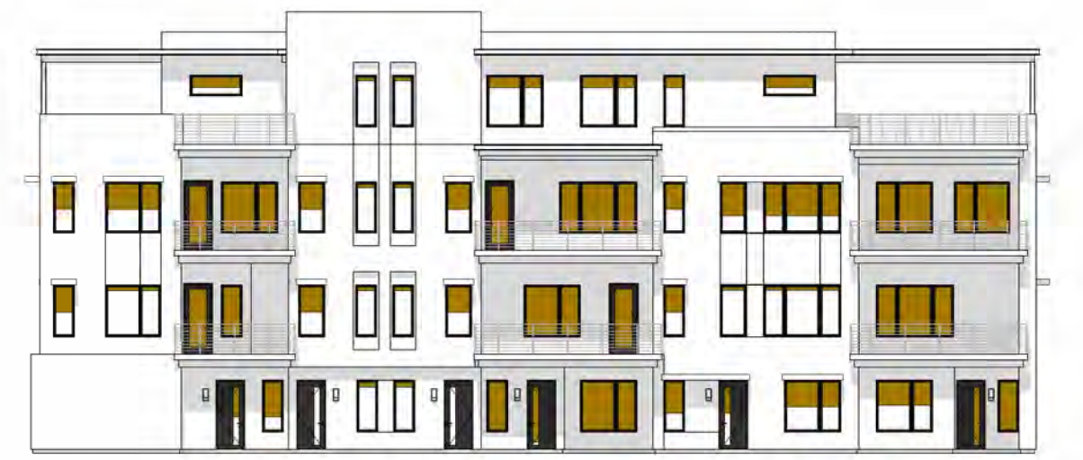
N TOTAL GLAZING: 1174.3 SF SHADED GLAZING: 697.3 SF
