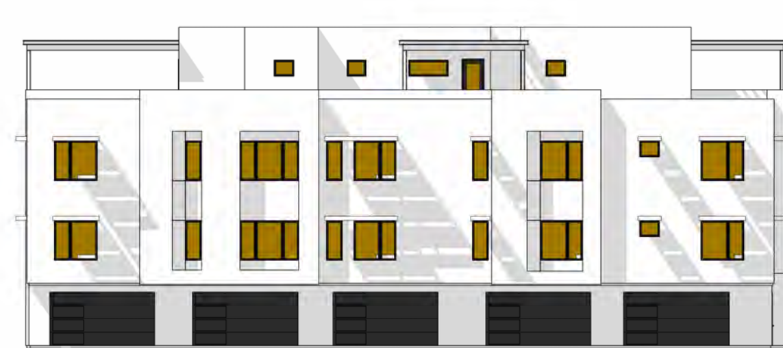
L TOTAL GLAZING: 570.1 SF SHADED GLAZING: 556.8 SF
