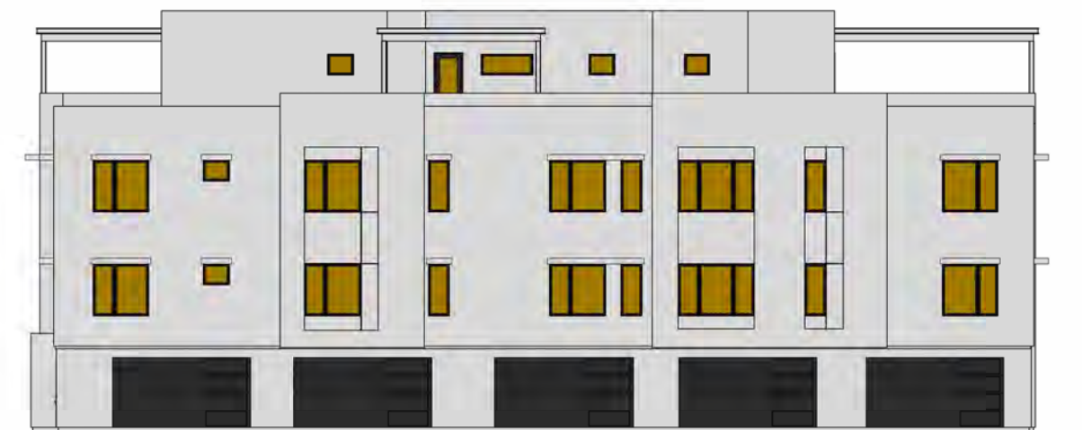
I TOTAL GLAZING: 570.1 SF SHADED GLAZING: 570.1 SF
