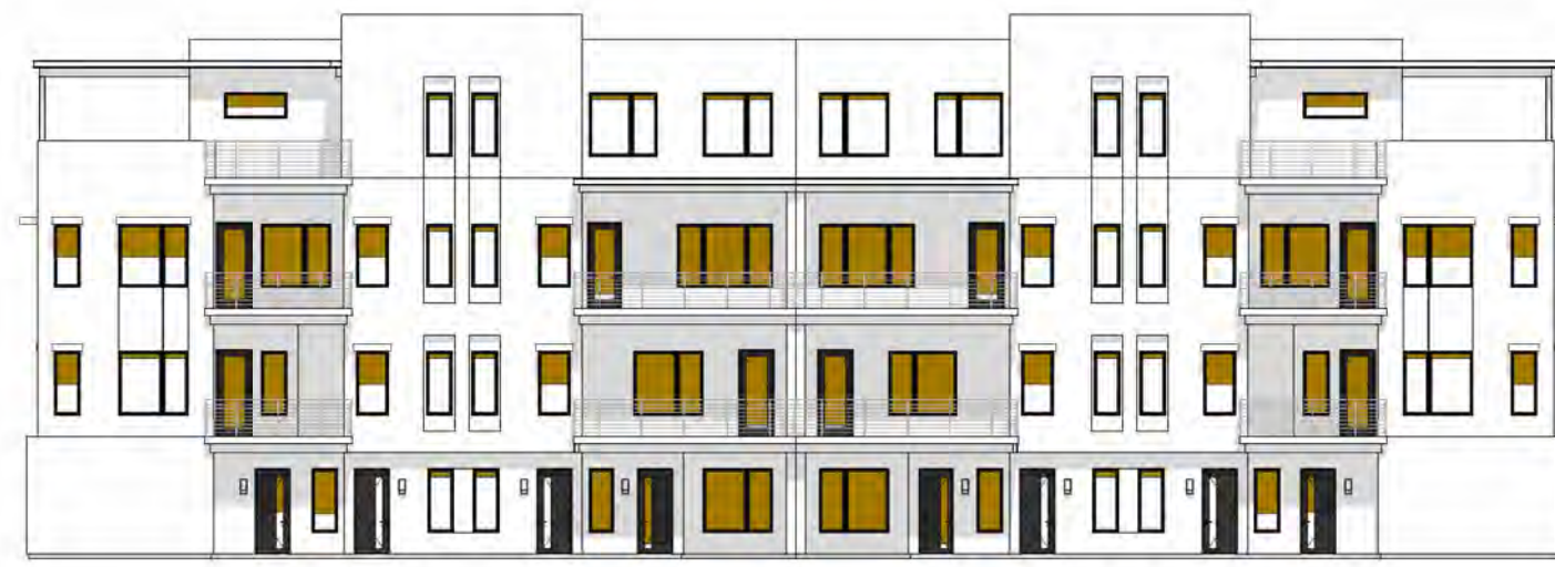
G TOTAL GLAZING: 1416.3 SF SHADED GLAZING: 774.3 SF
