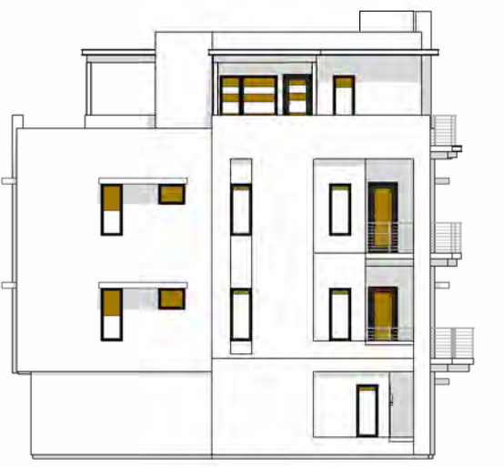
C TOTAL GLAZING: 209.5 SF SHADED GLAZING: 92.1 SF
