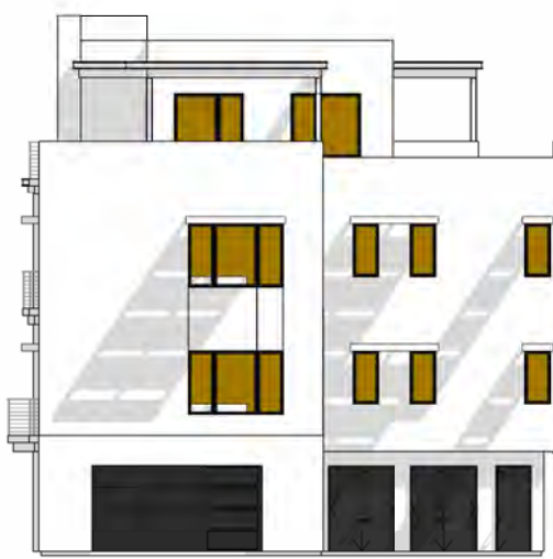
H TOTAL GLAZING: 256.7 SF SHADED GLAZING: 243.4 SF
