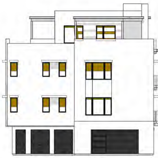
D TOTAL GLAZING: 256.7 SF SHADED GLAZING: 110.0 SF
