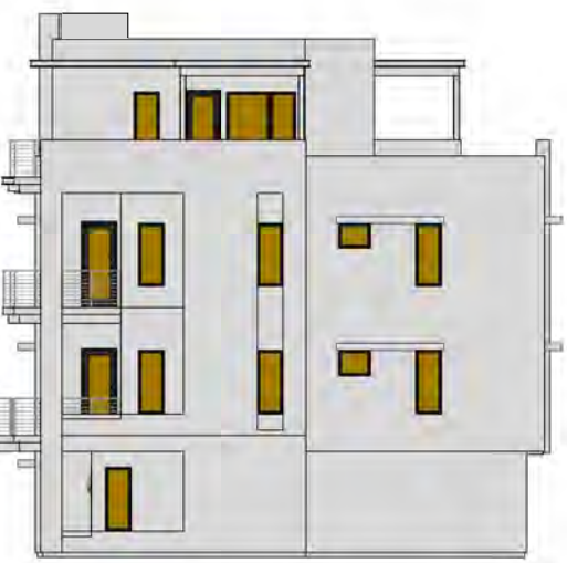
L TOTAL GLAZING: 209.5 SF SHADED GLAZING: 209.5 SF
