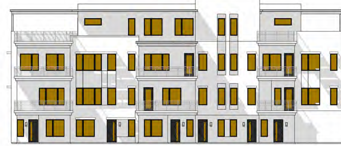
C TOTAL GLAZING: 1174.3 SF SHADED GLAZING: 1171.8 SF
