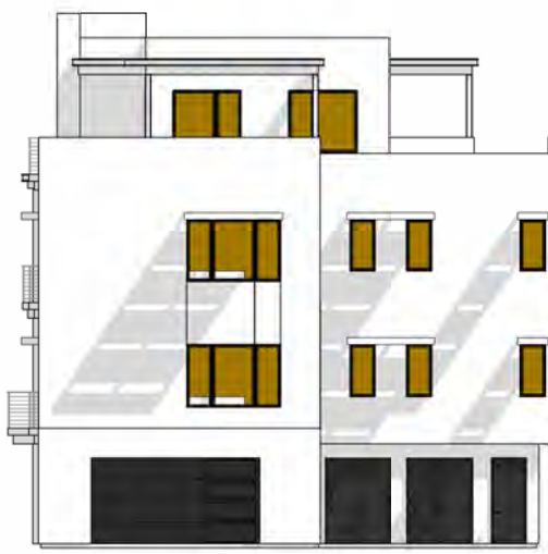
G TOTAL GLAZING: 256.7 SF SHADED GLAZING: 243.4 SF
