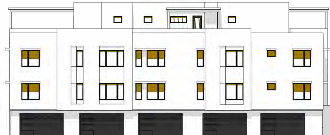
F TOTAL GLAZING: 570.1 SF SHADED GLAZING: 204.1 SF
