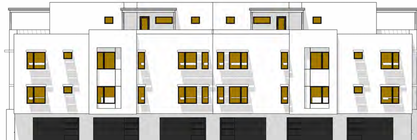
G TOTAL GLAZING: 697.7 SF SHADED GLAZING: 633.3 SF
