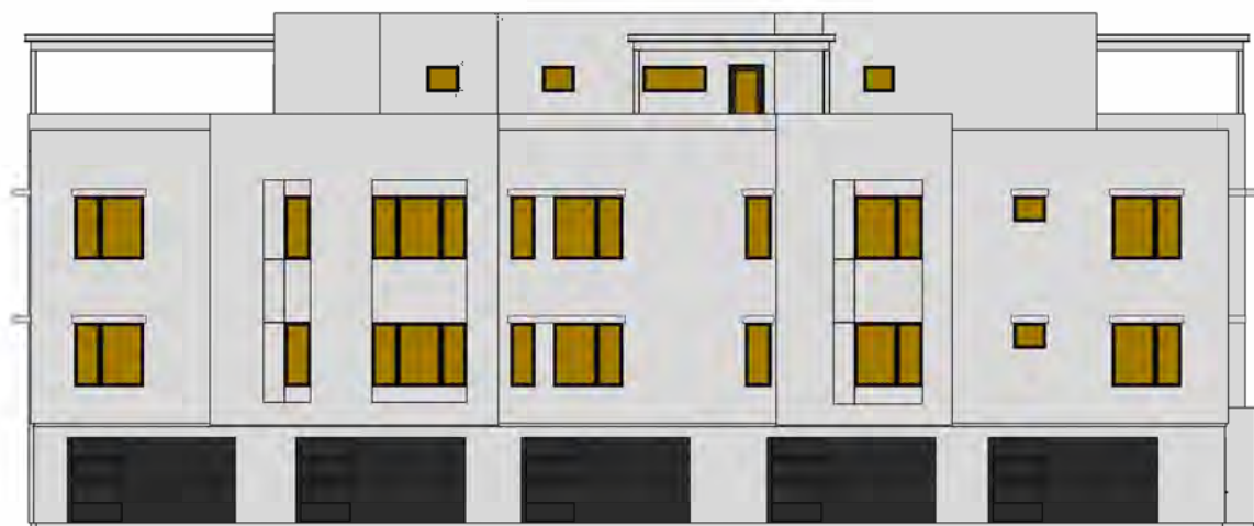
F TOTAL GLAZING: 570.1 SF SHADED GLAZING: 570.1 SF
