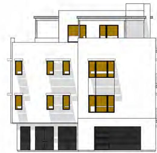
J TOTAL GLAZING: 256.7 SF SHADED GLAZING: 209.5 SF
