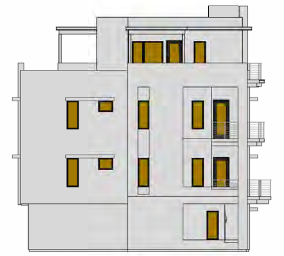
C TOTAL GLAZING: 209.5 SF SHADED GLAZING: 209.5 SF
