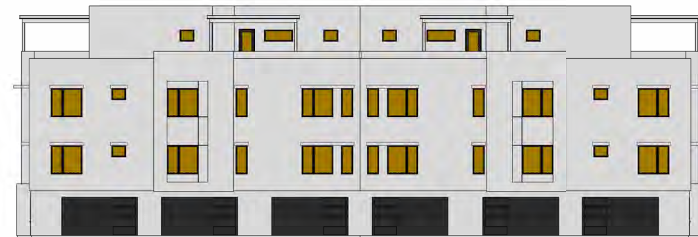
H TOTAL GLAZING: 697.7 SF SHADED GLAZING: 697.7 SF
