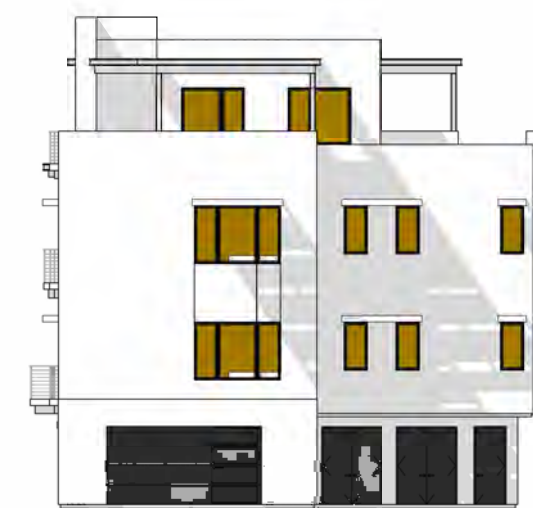
I TOTAL GLAZING: 256.7 SF SHADED GLAZING: 247.7 SF
