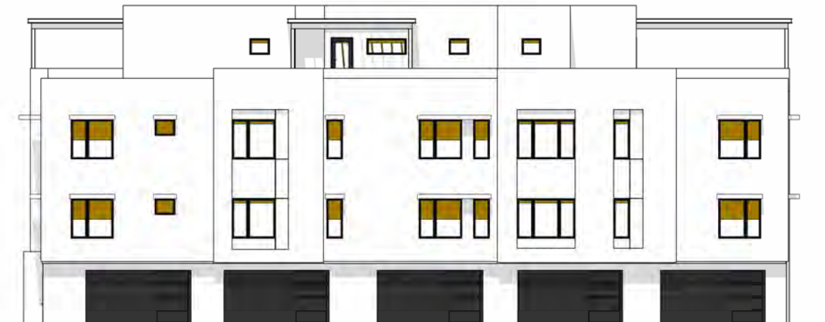
I TOTAL GLAZING: 570.1 SF SHADED GLAZING: 204.1 SF
