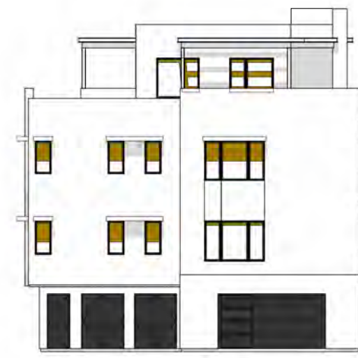
J TOTAL GLAZING: 256.7 SF SHADED GLAZING: 110.0 SF
