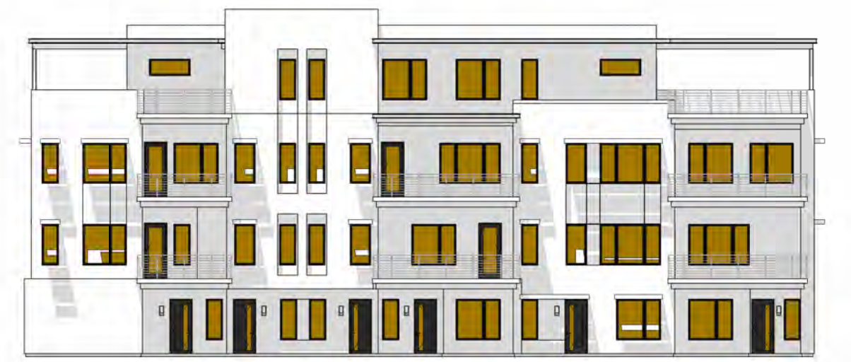
N TOTAL GLAZING: 1174.3 SF SHADED GLAZING: 1141.1 SF
