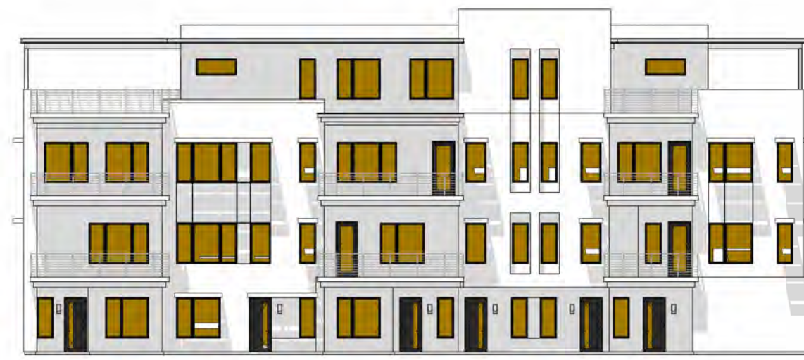
A TOTAL GLAZING: 1174.3 SF SHADED GLAZING: 1141.1 SF
