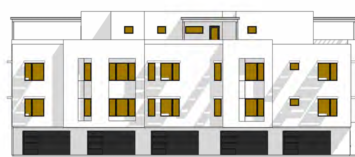
J TOTAL GLAZING: 570.1 SF SHADED GLAZING: 554.9 SF
