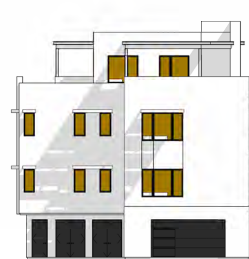
N TOTAL GLAZING: 256.7 SF SHADED GLAZING: 243.4 SF
