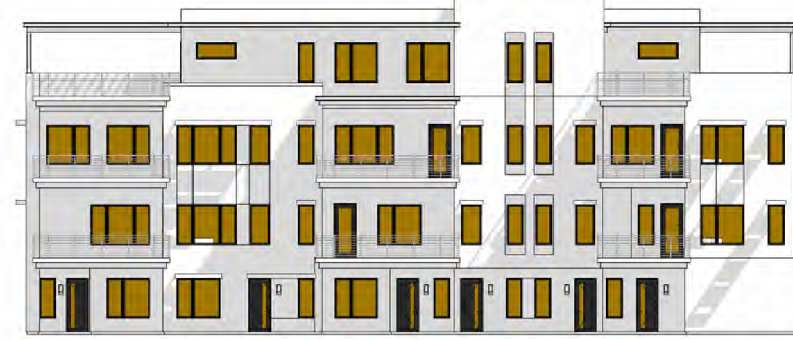
C TOTAL GLAZING: 1174.3 SF SHADED GLAZING: 1164.9 SF
