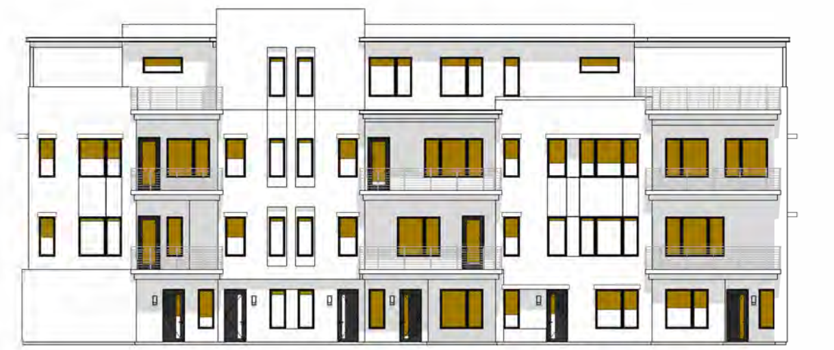
F TOTAL GLAZING: 1174.3 SF SHADED GLAZING: 686.5 SF
