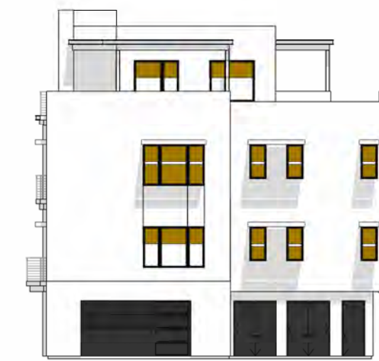
H TOTAL GLAZING: 256.7 SF SHADED GLAZING: 170.3 SF
