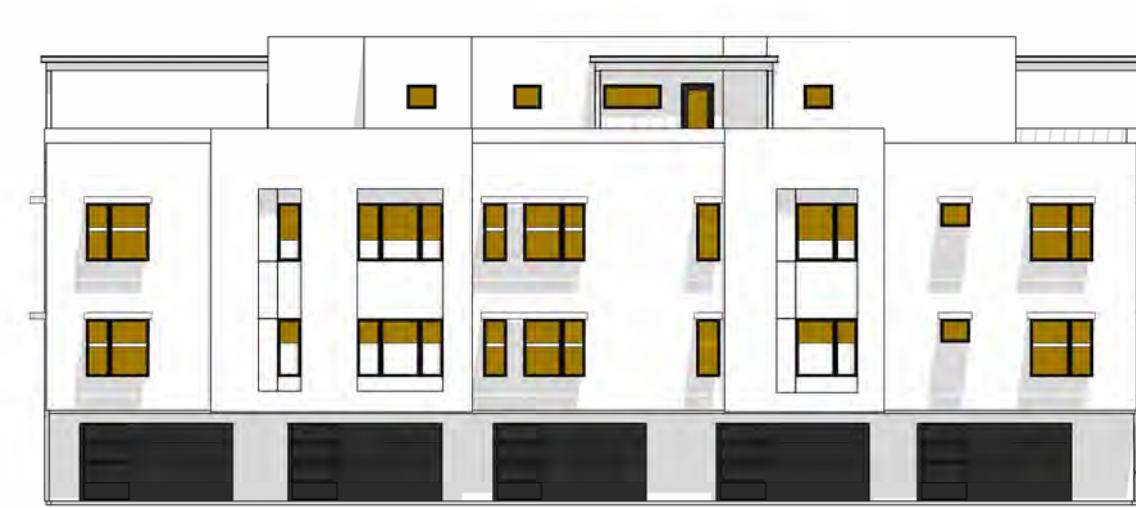
J TOTAL GLAZING: 570.1 SF SHADED GLAZING: 450.8 SF
