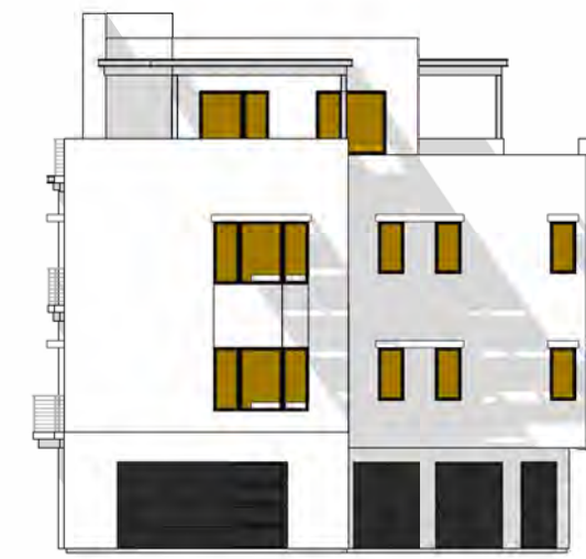
G TOTAL GLAZING: 256.7 SF SHADED GLAZING: 247.7 SF
