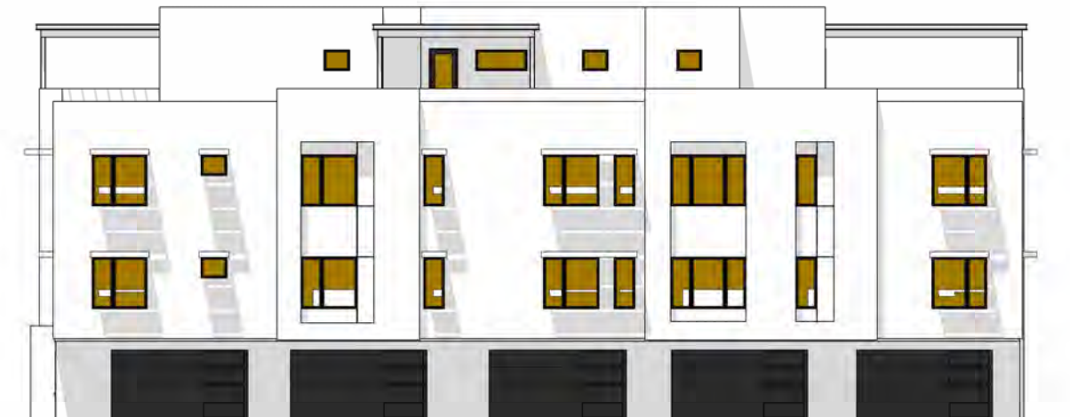
I TOTAL GLAZING: 570.1 SF SHADED GLAZING: 508.1 SF
