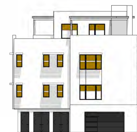
N TOTAL GLAZING: 256.7 SF SHADED GLAZING: 170.3 SF
