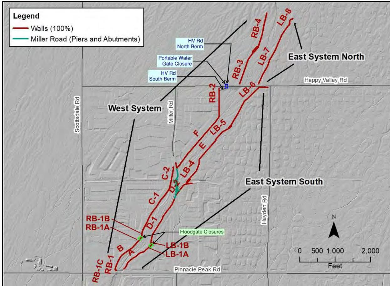
Figure 5-7. Levee Systems in the Natural Valley Procedure FLO-2D Modeling
