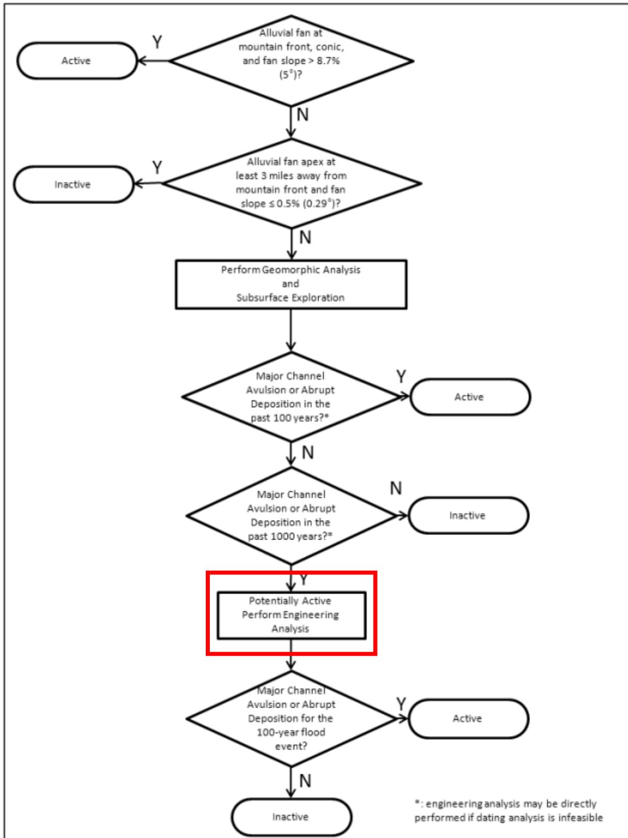
Figure 6-1. Flowchart for Stage 2 Determination of Active Alluvial Fan, from (FCDMC, 2014)
