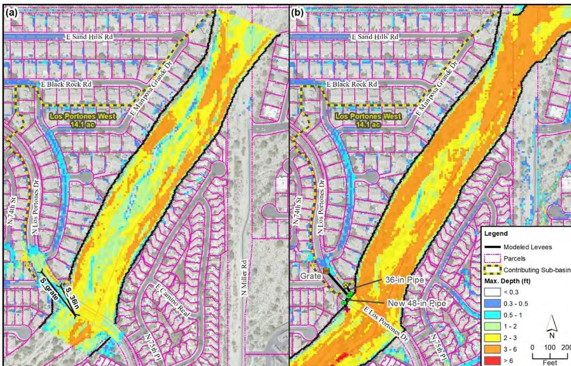
Figure 5-6. Comparison of (a) Existing and (b) Proposed Conditions on the West Side of Los Portones Drive
