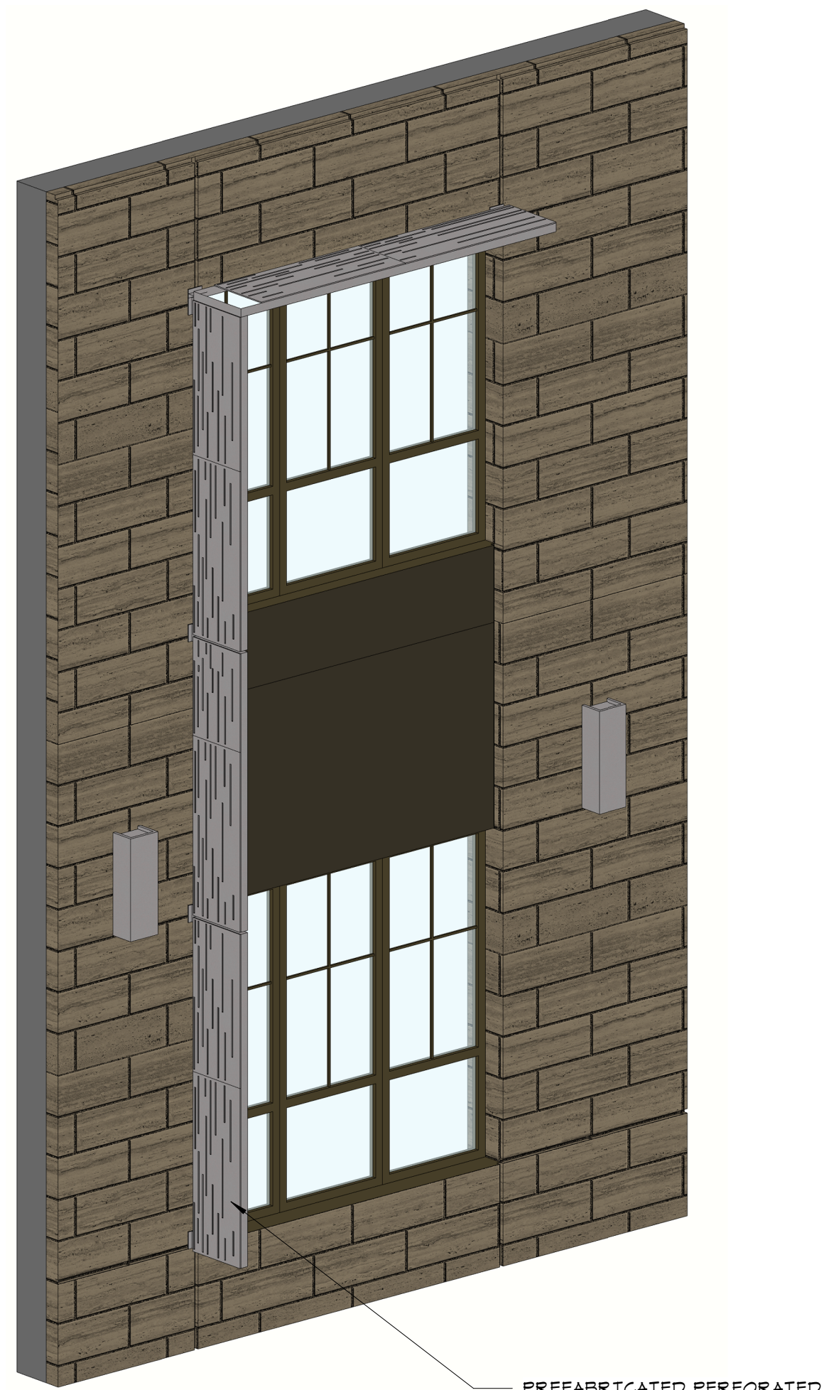
SUNSHADE ELEMENT AT SOUTH FACADE
