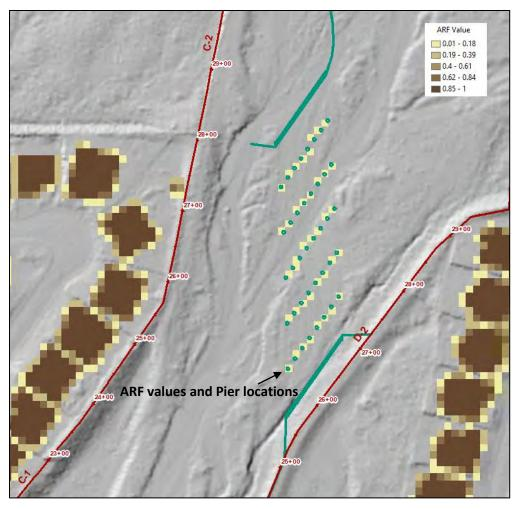
Figure 5-3. Schematic of Miller Road Piers and ARF Values
