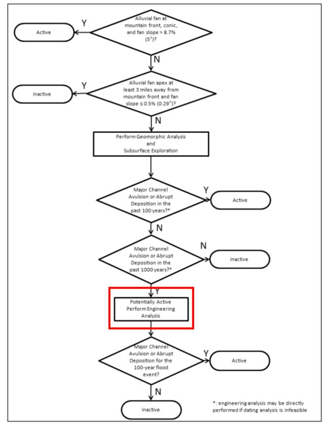
Figure 6-1. Flowchart for Stage 2 Determination of Active Alluvial Fan, from (FCDMC, 2014)
