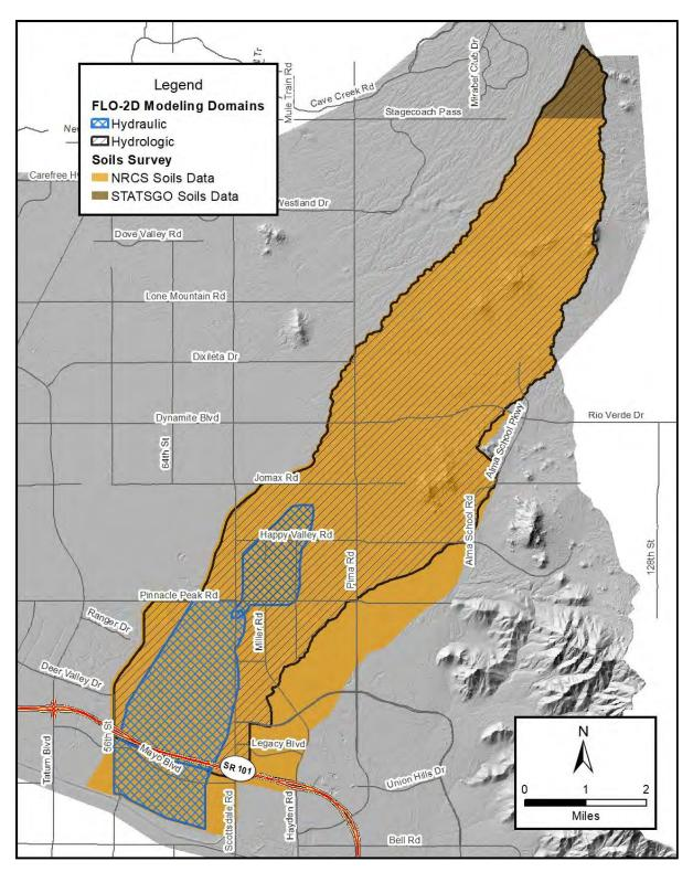
Figure 4-2. Soil Survey Coverage over the FLO-2D Model Domain
