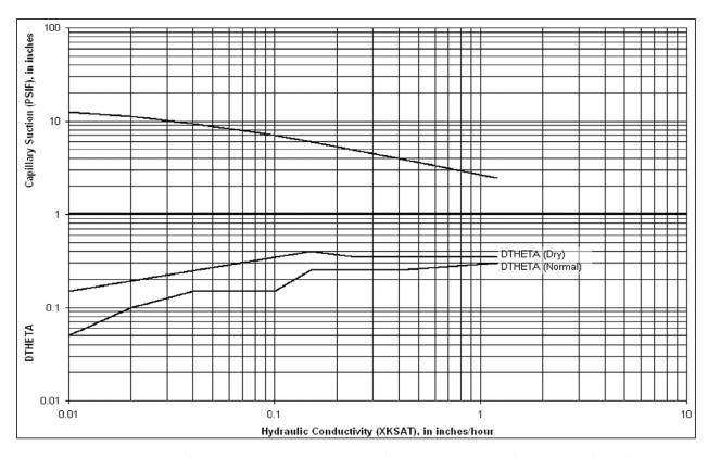
Figure 4-4. Values of PSIF and DTHETA as a Function of XKSAT, Reproduced from FCDMC (2018a).
