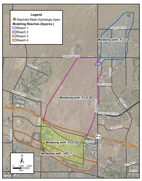
Figure 5-1. Hydraulic Modeling Reaches
