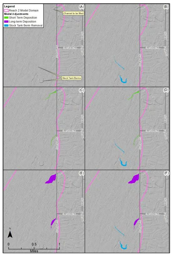
Figure 6-2. Spatial Locations of Model Adjustments for Avulsion Models: (A) 2016/2019 Topography, (B) 2016/2019 Topography with Stock Tank Removed, (C) 2016/2019 Topography with Short-term Deposition, (D) 2016/2019 Topography with Short-term Deposition and Stock Tank Removed, (E) 2016/2019 Topography with Long-term Deposition, and (F) 2016/2019 Topography with Long-term Deposition and Stock Tank Removed
